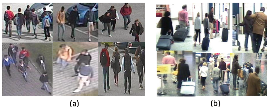
Fig. 6.3 Some example images from people group datasets: (a) OGRE dataset (b) Ilids-group dataset. One can note the challenging viewpoint variation and the resulting variations in relative positions of individuals as well as partial occlusions by objects, the image border or among individuals
