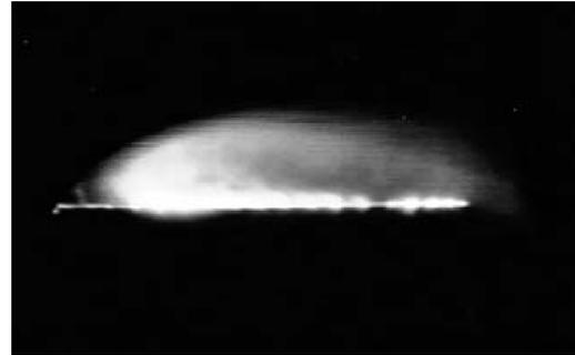
**Figure 2.14:** Flow pattern from the laser light visualization on the free end surface [ROH 03]
