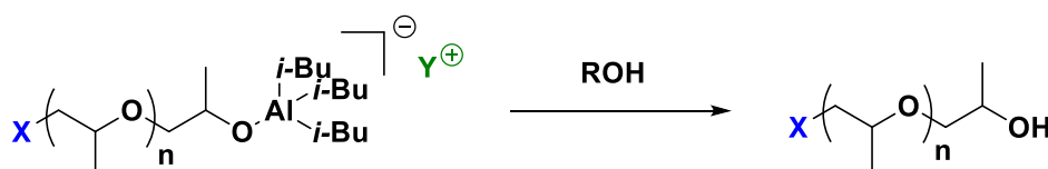
Scheme 13. AROP of propylene oxide in presence of i\text{-Bu}_3\text{Al} as activator proceeding by AMM.
