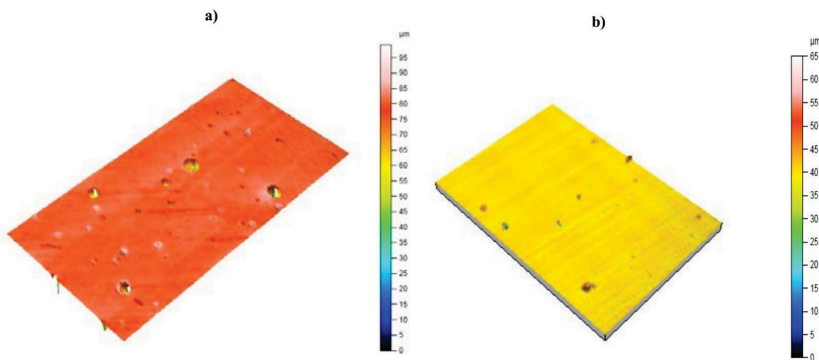
**Figure 1-14** Surface topography of cross section showing porosity of epoxy/amine networks containing a) 9 wt% and b) 12 wt%.<sup>110</sup>
