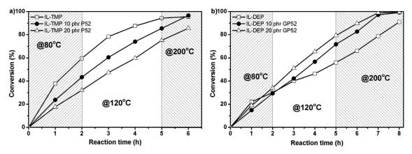
Figure 3-5 Epoxide group conversion as a function of curing time of epoxy/IL networks ( $\square$ ) modified by 10 phr ( $\bullet$ ) and 20 phr ( $\Delta$ ) CSR and cured with a) IL-TMP and b) IL-DEP.
