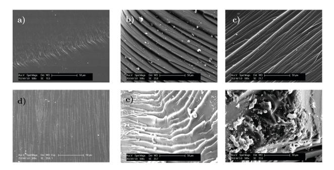
**Figure 4-11** Fracture surface of unmodified (a,d) and CA-modified epoxy/IL networks containing 10 phr (b,e) and 20 phr (c,f) of CA cured with IL-DCA (a,b,c)and IL-TMP (d,e,f).
