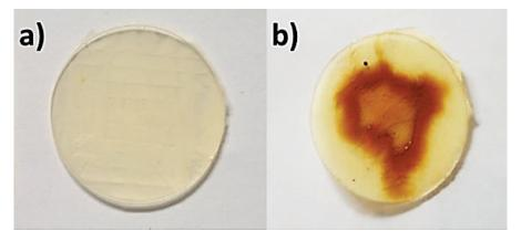
**Figure 2-3** Samples of epoxy prepolymer containing different amount of IL-TMP of (a) 10 phr and (b) 20 phr (Exudation of IL on the surface of samples with color change due to the oxidation).
