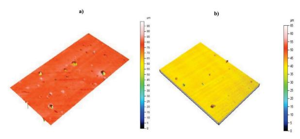
Figure 1-14 Surface topography of cross section showing porosity of epoxy/amine networks containing a) 9 wt% and b) 12 wt%.
