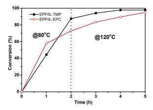
**Figure 2-26** Epoxy conversion as a function of curing time of EPP/IL-TMP (■) and EPP/IL-EPC (O) systems.
