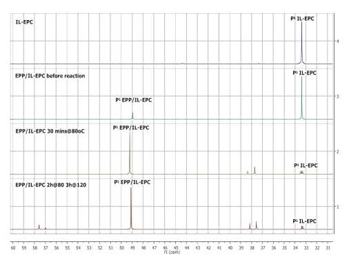
**Figure 2-30**  $^{31}$ P NMR of IL-EPC and EPP/IL-EPC systems before the reaction and after 30 minutes and 5 h of curing process.
