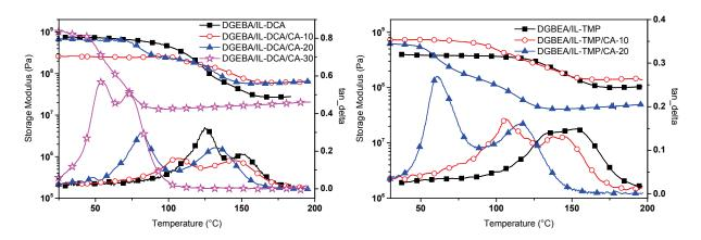
**Figure 4-8** DMA analysis of (■) unmodified, CA-modified epoxy networks containing 10 phr (O), 20 phr (▲), 30 phr of CA (☆) cured by IL-DCA (left) and IL-TMP (right).
