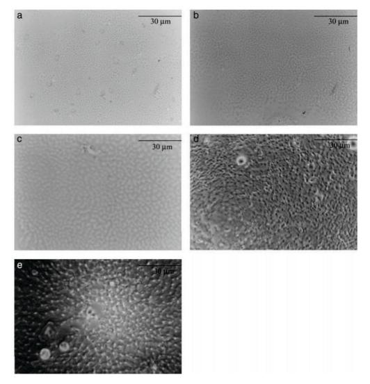
Figure 1-23 Optical micrographs of PPE-modified epoxy blends (30phr) cured for different times at 180  $^{\circ}$ C showing the spinodal decomposition.  $^{145}$
