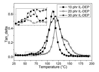
**Figure 2-11** Loss factor  $\tan\delta$  as a function of temperature of epoxy/phosphate ionic liquid IL-DEP at different contents: 10 phr ( $\blacksquare$ ), 20 phr ( $\bigcirc$ ) and 30 phr ( $\star$ ).
