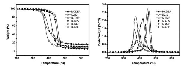
Figure 2-18 Weight loss as a function of temperature (TGA, DTGA) of epoxy networks: MCDEA ( $\blacksquare$ ), Jeffamine D230 (O), IL-TMP ( $\Delta$ ), IL-EPC ( $\spadesuit$ ), IL-DEP ( $\Rightarrow$ ) and IL-EHP ( $\blacktriangleleft$ ) (heating ramp 20 K.min<sup>-1</sup>, N<sub>2</sub> atmosphere).
