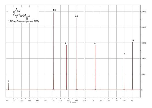
Figure S2-2 <sup>13</sup>C NMR of 1,2-epoxy 3-phenoxy propane (EPP).
