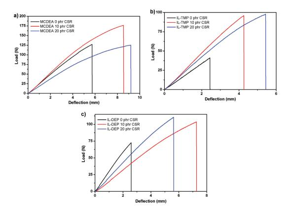
**Figure S2-5** Load-deflection curves of epoxy networks modified by CSR using a) MCDEA, b) IL-TMP and c) IL-DEP (2 mm.min<sup>-1</sup>).
