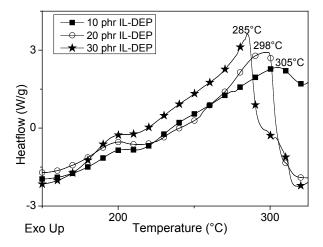
**Figure 2-5** DSC thermograms of epoxy/ 10phr IL-DEP (■), epoxy/ 20phr IL-DEP (O) and epoxy/ 30phr IL-DEP (★).
