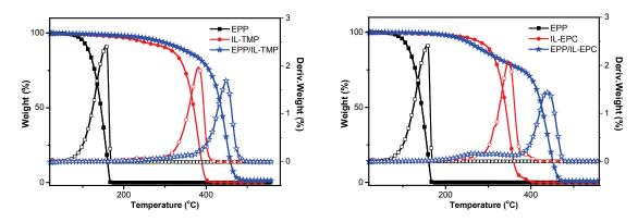
Figure 2-24 TGA ( $\blacksquare$ , $\bullet$ , $\star$ ) and DTGA ( $\blacksquare$ , $\bigcirc$ , $\diamond$ ) curves of EPP ( $\blacksquare$ , $\blacksquare$ ), neat IL ( $\bullet$ , $\bigcirc$ ) and EPP/ILs ( $\star$ , $\diamond$ ) for EPP/IL-TMP (left) and EPP/IL-EPC (right) systems.
