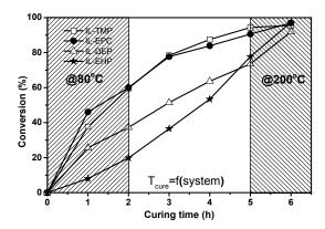
**Figure 2-15** Epoxide group conversion as a function of curing time calculated from FT-IR spectra of different epoxy/IL systems during cure (see Table 2-2 for curing schedules which differ for each reactive system).
