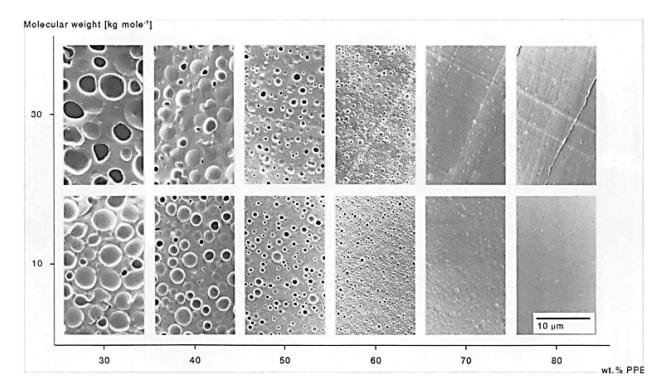
**Figure 1-22** Morphology of epoxy/PPE blends with PPE molar mass of 10 and 30 kg.mol<sup>-1</sup> and PPE content of 30-80 wt% after cooling from 200°C to room temperature observed by scanning electron microscopy.<sup>138</sup>
