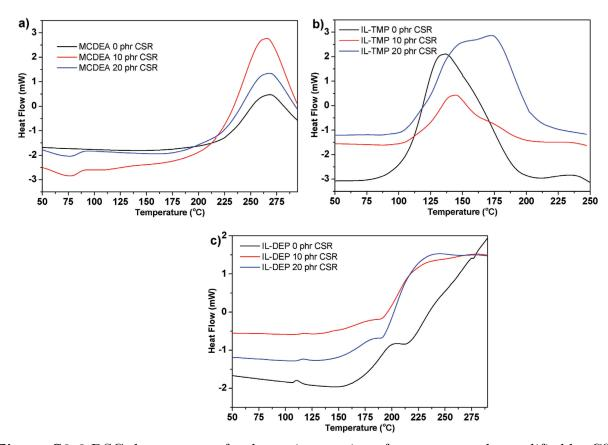
**Figure S3-2** DSC thermograms for dynamic scanning of epoxy networks modified by CSR using MCDEA (a), IL-TMP (b) and IL-DEP (c).
