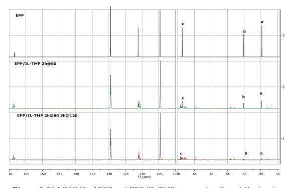
Figure 2-28  $^{\rm 13}{\rm C}$  NMR of EPP and EPP/IL-TMP system after 2h and 5h of curing.
