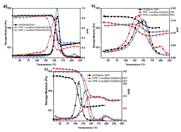
Figure 3-2 DMA analysis of ( $\blacksquare$ ) unmodified, ( $\bullet$ ) PPE-1-modified and ( $\updownarrow$ ) PPE-2-modified epoxy networked cured by a) MCDEA, b) IL-TMP and c) IL-DEP.
