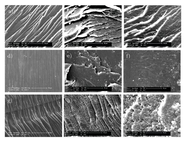
**Figure 3-4** Fracture surface of unmodified (a, d, g), modified by PPE-1 (b, e, h) and PPE-2 (c, f, i) modified epoxy/amine (a, b,c), epoxy/IL-TMP (d, e, f) and epoxy/IL-DEP (g, h,i) networks observed by SEM.
