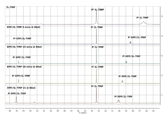
**Figure 2-29** <sup>31</sup>P NMR of IL-TMP and EPP/IL-TMP system after 5 minutes, 15 minutes, 30 minutes and 1 hour at 80 °C.
