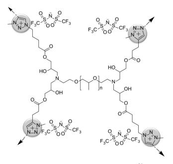
Figure 1-8 Crosslinked triazolium based epoxy-amine networks.<sup>94</sup>
