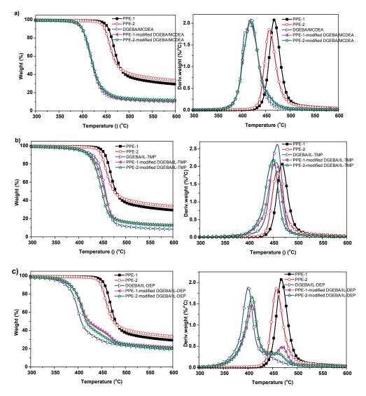
Figure 3-3 Weight loss as a function of temperature of neat PPE-1 (■), PPE-2 (O), unmodified epoxy networks (▷) and PPE-modified considering the addition of PPE-1 (◄) and PPE-2 (☆) cured by a) MCDEA, b) IL-TMP and c) IL-DEP.
