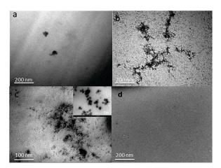
**Figure 1-10** TEM images of epoxy networks containing 10 phr of (a) Phos-DCA, (b) Phos-DBS, (c) Phos-TFSI and (d) without IL. 100
