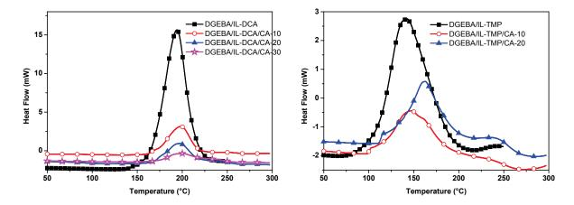
Figure 4-5 DSC thermogram of CA-modified epoxy/IL networks.
