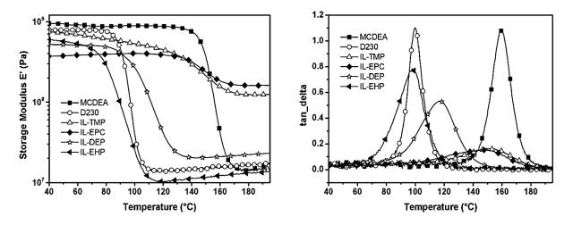
**Figure 2-19** Storage modulus E' and loss factor tan  $\delta$  as a function of temperature of DGEBA-based networks cured with different types of curing agent: MCDEA ( $\blacksquare$ ), Jeffamine D230 (O), IL-TMP ( $\Delta$ ), IL-EPC ( $\diamondsuit$ ), IL-DEP ( $\diamondsuit$ ), and IL-EHP ( $\blacktriangleleft$ ) at 1Hz.
