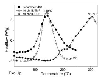
**Figure 2-4** DSC thermograms of epoxy/Jeffamine D400 (■), epoxy/ 10 phr IL-TMP (O) and epoxy/ 10 phr IL-DEP ( $\star$ ).
