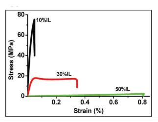
Figure 1-11 Tensile stress-strain curves of hard thermoset (black curve) showing perfectly brittle fracture at 10 % IL, plastic thermosets showing ductile behavior at 30 % of IL (red curve) and S-shaped curves of elastomeric thermosets at 50 % IL (green curve). $^{102}$
