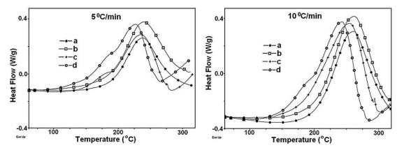
**Figure 1-9** DSC thermograms of DGEBA/MCDEA networks as a function of heating rate and IL content (a) 0, (b) 1, (c) 2.5 and (d) 5 phr of IL.<sup>97</sup>
