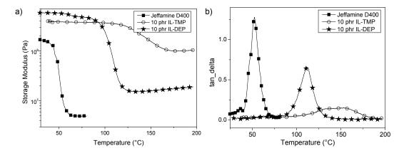
**Figure 2-10** Storage Modulus E' (a) and loss factor  $\tan\delta$  (b) as a function of temperature of DGEBA systems with different types of curing agent: Jeffamine ( $\blacksquare$ ), 10 phr IL-TMP (O) and 10 phr IL-DEP ( $\star$ ) from DMA with measurement rate of 3 °C.min<sup>-1</sup>.
