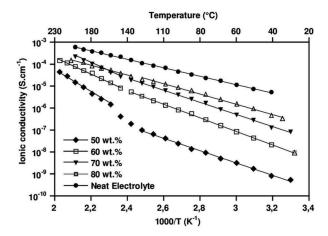
Figure 1-12 Ionic conductivity of gel polymer electrolyte with different amounts of Phos-TMP with 0.2 M of lithium salt.<sup>105</sup>
