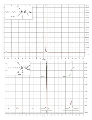
Figure S2-4 <sup>31</sup>P NMR of IL-EPC, IL-TMP and IL-DEP.
