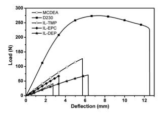
**Figure 2-21** Load-deflection curves of epoxy/different curing agents: MCDEA (O), Jeffamine D230 ( $\blacksquare$ ), IL-TMP ( $\Delta$ ), IL-EPC ( $\spadesuit$ ) and IL-DEP ( $\star$ ) (2 mm.min<sup>-1</sup>).
