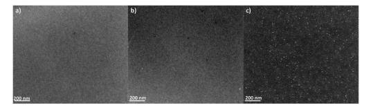
**Figure 1-17** TEM micrographs of the epoxy networks cured with (a) 5 phr, (b) 10 phr and (c) 30 phr of phosphonium dicyanamide ILs.<sup>124</sup>
