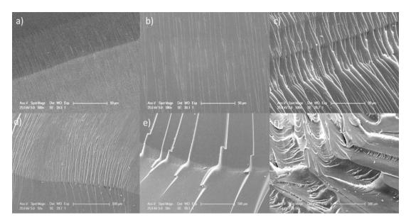
**Figure 2-20** Fractured surfaces of epoxy networks cured with IL-EPC (a), IL-TMP (b), and MCDEA (c) at magnification of  $\times 500$  (up) and MCDEA (d), IL-DEP (e) and D230 (f) at magnification of  $\times 50$  (down).
