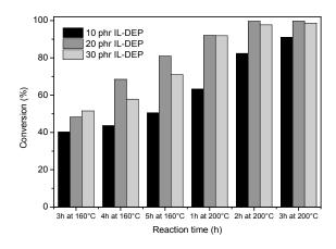
**Figure 2-7** Conversion of epoxide groups versus reaction time of (a) epoxy/different curing agents and (b) epoxy/different amounts of IL-DEP.
