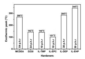
**Figure 2-14** Reaction enthalpy peak temperature (DSC, 10 K.min<sup>-1</sup>) of different epoxy reactive systems.
