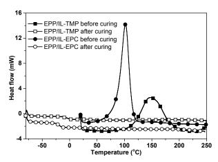
Figure 2-23 DSC thermogram of EPP/IL-TMP ( $\blacksquare$ , $\blacksquare$ ) and EPP/IL-EPC ( $\bullet$ , $\bigcirc$ ) systems: before ( $\blacksquare$ , $\bullet$ ) and after the curing procedure ( $\blacksquare$ , $\bigcirc$ ).
