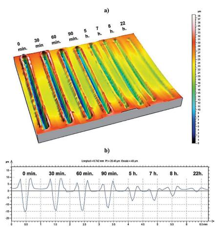
**Figure 1-13** Surface topography and cross section profiles of epoxy/amine networks containing 12 wt% of IL showing the evolution of wear track as a function of time. <sup>110</sup>
