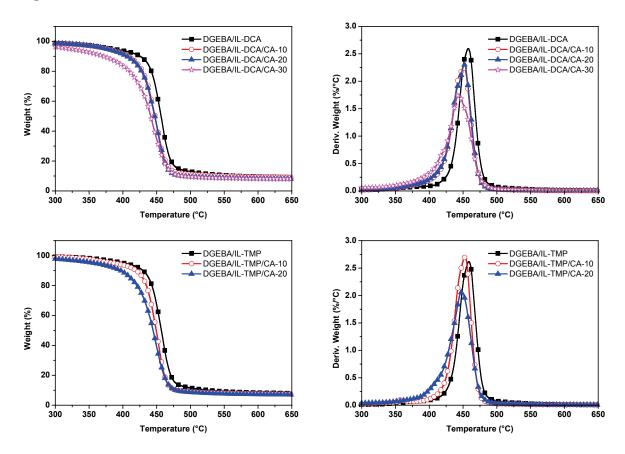
**Figure 4-9** Weight loss as a function of temperature (TGA, DTGA) (■) unmodified and CA-modified epoxy networks containing 10 phr (O), 20 phr (▲), 30 phr of CA (☆) cured by IL-DCA (up) and IL-TMP (down).
