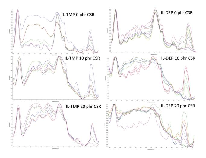
**Figure S3-3** Evolution of FTIR spectra with curing time of epoxy networks modified by CSR using IL-TMP (left) and IL-DEP (right).
