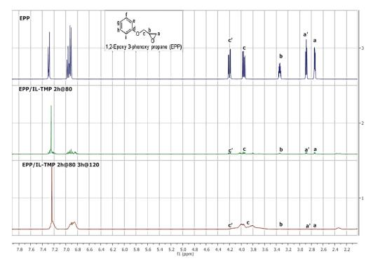
Figure 2-27  $^1$ H NMR of EPP and EPP/IL-TMP system after 2h and 5h of curing.
