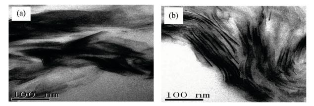
**Figure 1-15** IL-modified clay dispersion in epoxy nanocomposite cured with a) imidazoles (intercalation) and b) anhydride (exfoliation).<sup>113</sup>
