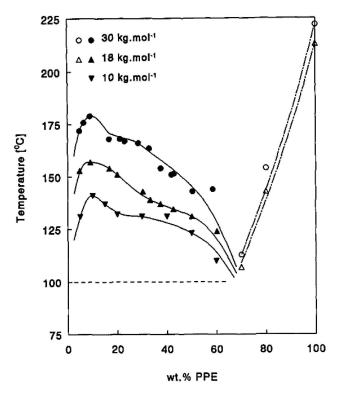
Figure 1-21 Phase diagram of epoxy/PPE blends including (—) cloud point curve, (-·-) calculated  $T_g$  lines and (——)  $T_g$  due to thermoreversible gelation.<sup>138</sup>
