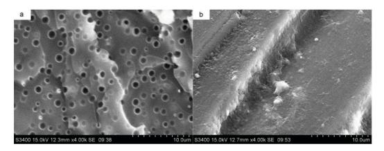
**Figure 1-28** SEM micrographs of the fracture surface of DGEBA based epoxy networks cured with a) MBCBE showing the cavities and b) Phenalkamines with no phase separation.<sup>200</sup>
