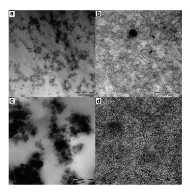
**Figure 1-16** Epoxy-silica hybrids: (a) without ILs and those formed in the presence of (b) methyl sulfonate based IL,(c) tetrafluoroborate based IL and (d) tetrafluoroborate based IL and hydrochloric acid.<sup>115</sup>
