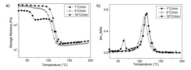
**Figure 2-12** Storage Modulus E' (a) and loss factor tanδ (b) as a function of temperature of epoxy/10 phr IL-DEP at different DMA measuring velocity: 1 °C.min<sup>-1</sup> (■), 3 °C.min<sup>-1</sup> (O) and 10 °C.min<sup>-1</sup> (★).
