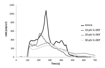
Figure 5-1 Heat release rate curves for epoxy resins in cone calorimeter test (heat flux 35 kW/m<sup>2</sup>).
