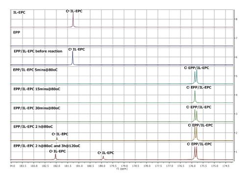
**Figure 2-33** <sup>13</sup>C NMR of IL-EPC and EPP/IL-EPC systems before the reaction and after 30 mins and 5 hours of curing (chemical shift from 173 to 184 ppm).
