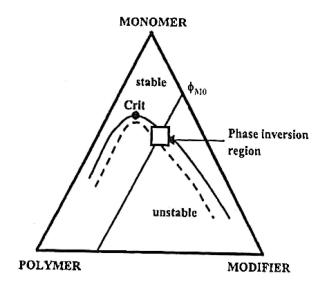
**Figure 1-20** Ternary phase diagram of TS/TP blends formed by chainwise polymerization (Crit. = critical point). 129
