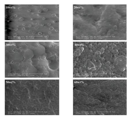
**Figure 1-24** SEM micrographs of PPE modified epoxy networks cured by imidazole with different PPE content (10-60 wt%).<sup>135</sup>
