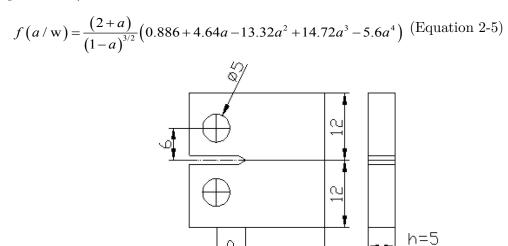
Figure 2-2 Compact Tension specimen configuration.
