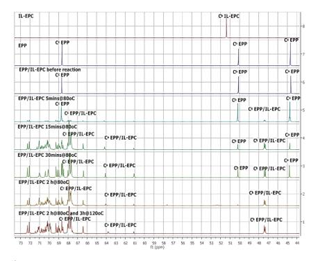
**Figure 2-32** <sup>13</sup>C NMR of IL-EPC, EPP and EPP/IL-EPC systems before the reaction and after 5, 15, 30 mins, 2 hours and 5 hours of curing (chemical shift from 44 to 74 ppm).
