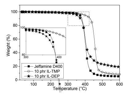
Figure 2-8 Evolution of weight loss as a function of temperature (TGA) of epoxy networks with different curing agents: Jeffamine D400 ( $\blacksquare$ ), 10 phr IL-TMP ( $\bigcirc$ ) and 10 phr IL-DEP ( $\star$ ).
