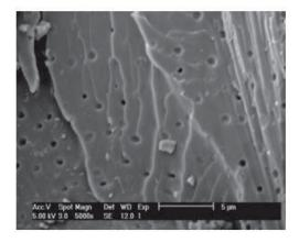
**Figure 1-25** Shear yielding mechanism of rubber-modified epoxy networks indicated by the formation of furrows running almost parallel to the principal tensile.<sup>161</sup>
