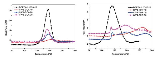
**Figure 4-2** DSC curves (10 K.min<sup>-1</sup>, under nitrogen) of different epoxy/IL reactive systems containing IL-DCA (left) and IL-TMP (right).
