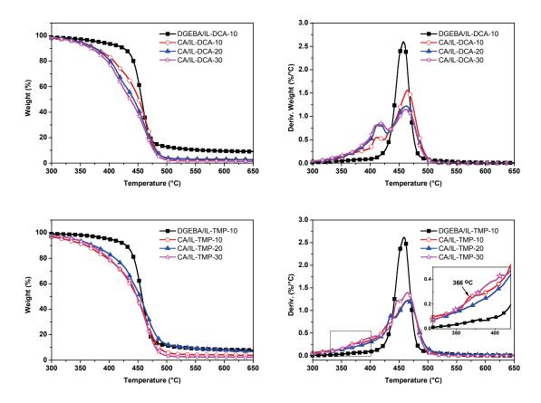
**Figure 4-4** Weight loss as a function of temperature (TGA, DTGA) of epoxy/IL networks cured with IL-DCA (up) and IL-TMP (down): at left, evolution of weight and at right, derivative of weight loss as a function of temperature.
