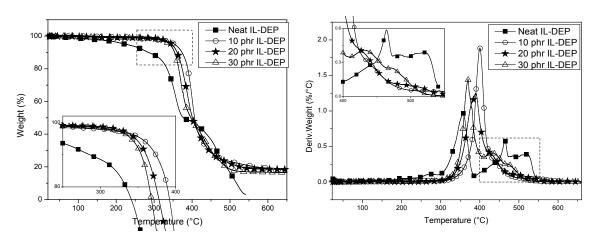
**Figure 2-9** Evolution of weight loss as a function of temperature (TGA, DTGA) of neat ionic liquid IL-DEP ( $\blacksquare$ ) and epoxy/IL-DEP networks: 10 phr ( $\bigcirc$ ), 20 phr ( $\star$ ) and 30 phr ( $\triangle$ ).
