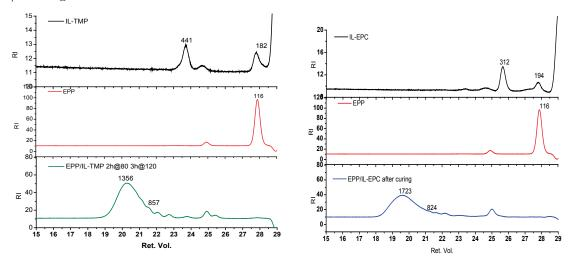
**Figure 2-25** SEC analysis for IL, EPP, EPP/ILs systems after curing for IL-TMP (left) and IL-EPC (right).
