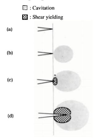
**Figure 1-26** Toughening mechanism of CSR-modified epoxy networks summarized by four steps: a) initial starter crack; b) formation of cavitation zone; c) formation of initial shear-yielded plastic zone and d) propagation of crack under shear yielding. <sup>162</sup>
