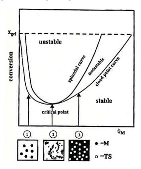
**Figure 1-19** Conversion vs composition transformation diagram type LCTS for a TS/TP blends in case of stepwise polymerization (M: TP phase).<sup>129</sup>
