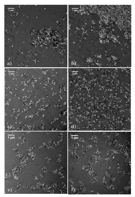
**Figure 3-6** TEM image of epoxy networks modified by 10 (a, c, e) and 20 phr (b, d, f) of CSR using MCDEA (a, b), IL-TMP (c, d) and IL-DEP (e, f).
