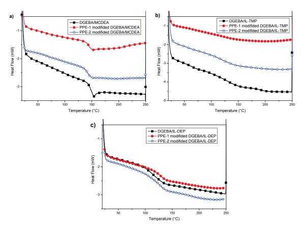
**Figure S3-1** DSC thermograph of ( $\blacksquare$ ) unmodified, ( $\bullet$ ) PPE-1-modified and (☆) PPE-2-modified epoxy networked cured by a) MCDEA, b) IL-TMP and c) IL-DEP.
