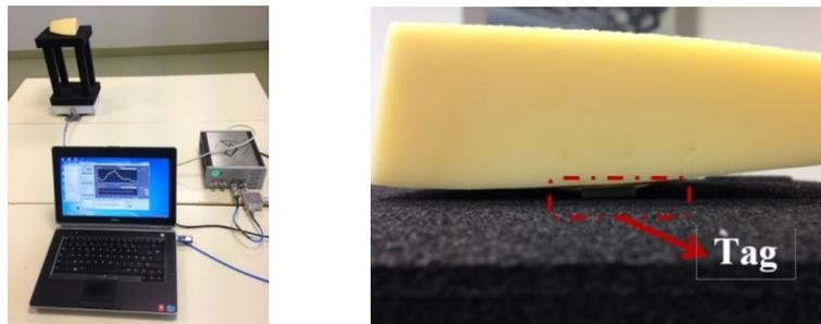
*Fig. 3. Read range measurement setup using Voyantic Tagformance.*
