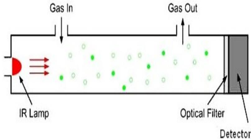
*Fig. 5. Non-Dispersive Infrared (NDIR) gas measurement system [12]*
