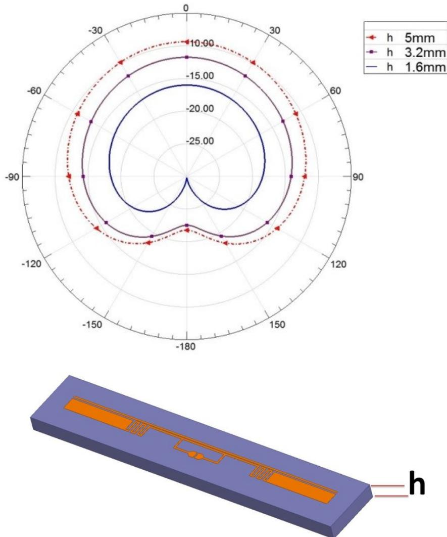
*Fig. 16. 3D model of simulated tag on cheese and a comparison between the gains of the tag (at  $\phi=90$  deg) simulated on FR4 substrates for 3 different thicknesses*
