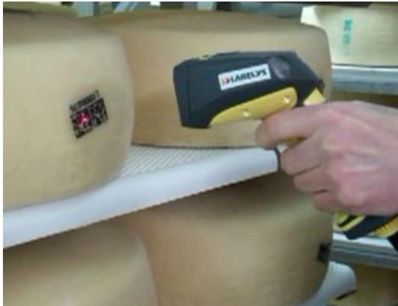
*Fig. 2. Cheese traceability system based on Barcodes [3]*
