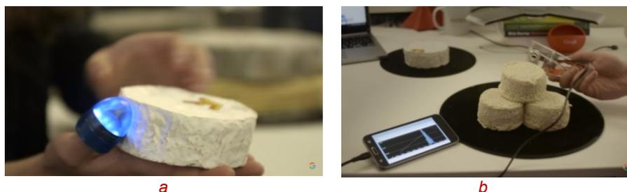
*Fig. 8. Google cheese master research project for monitoring cheese quality based on several types of sensors a) Optical sensor b) Ultrasound sensor [59]*
