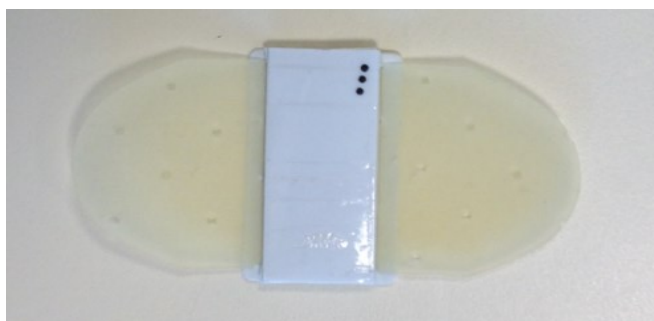
Fig. 1. a) Tag encapsulated between two layers of polypropylene b) tag sealed with resin before installation on cheese
