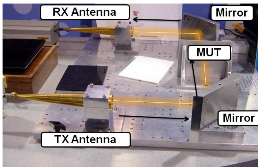
*Fig. 16. Measurement setup of free space quasi-optical system [42]*
