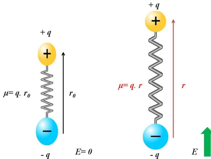
*Fig. 2. Atomic polarization mechanism where the ionic bonds stretch due to the applied field.*
