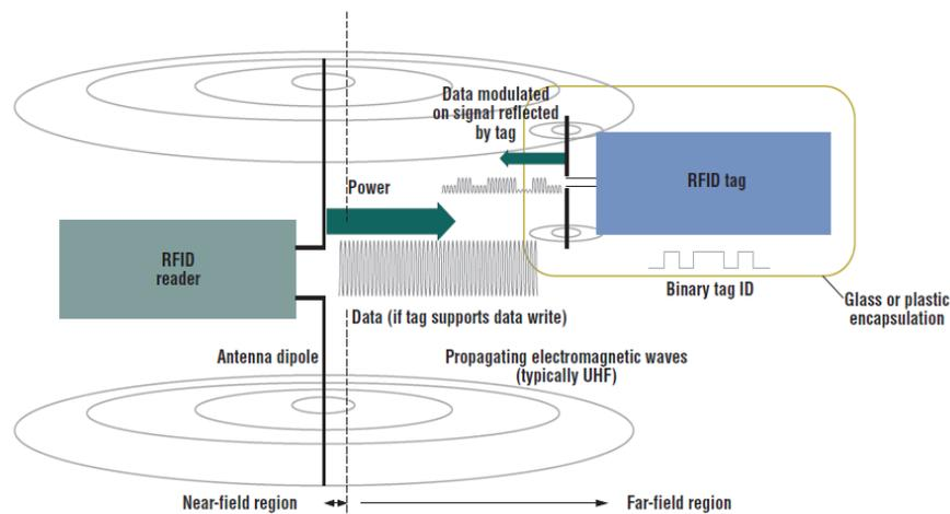
*Fig. 2. Principle of backscattering in Far-field RFID system [5].*
