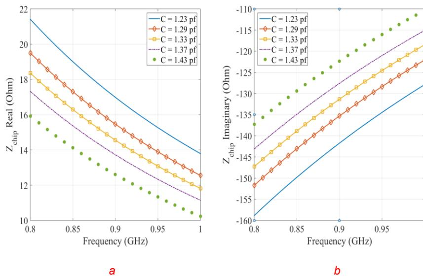
**Fig 5. Simulation results of Monza R6\_P chip impedance variation due to auto-tuning according to the datasheet RC model a) Real b) Imaginary**
