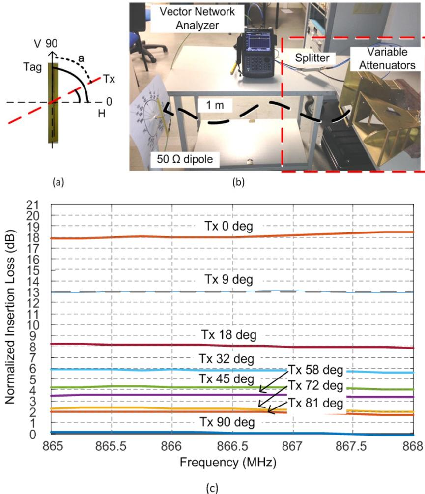
*Fig. 6. Measurement of the insertion loss between the proposed reader antenna configuration and a 50  $\Omega$  dipole centered at 867 MHz and placed in vertical position (90 degrees). The minimum insertion loss was realized for a transmitted polarization which corresponds to dipole orientation ( $\alpha = 0$  degree)). (a) angles definition. (b) Bench. (c) Measurement result.*
