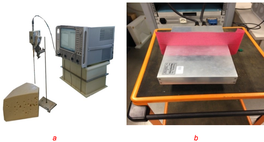
Fig. 4. Different characterization methods a) dielectric characterization of cheese using a coaxial probe b) characterization of thin sheets of casein in a resonant cavity
