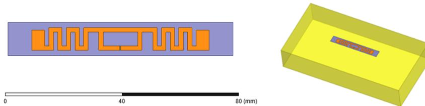
*Fig. 21. HFSS simulation model of PLA tag on cheese*
