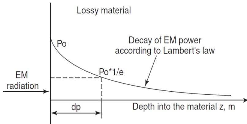
*Fig. 5. Penetration depth inside a lossy dielectric material. [6]*
