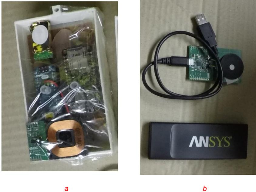
*Fig. 7. CO<sub>2</sub> sensor powered by coupling a) Rx coupling module connected to the sensor circuit b) Tx coupling module powered by a USB battery pack*
