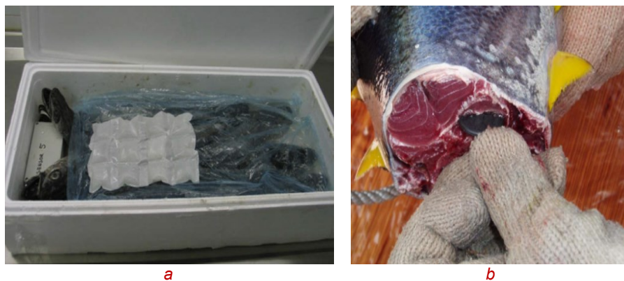
Fig.6. Different RFID system configurations for traceability in the fish sector a) RFID HF tag placed inside a polystyrene box with the fish for identification and temperature monitoring [39] b) RFID HF tag implanted into Tuna caudal fin root [40].
