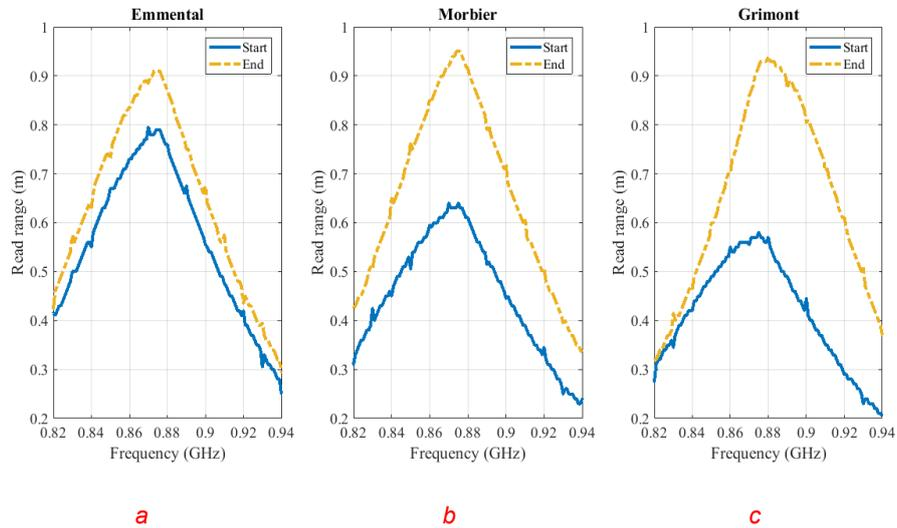
*Fig. 4. AK5 tag read range comparison between start and end of ripening for three types of cheese a) Emmental b) Morbier c) Grimont*
