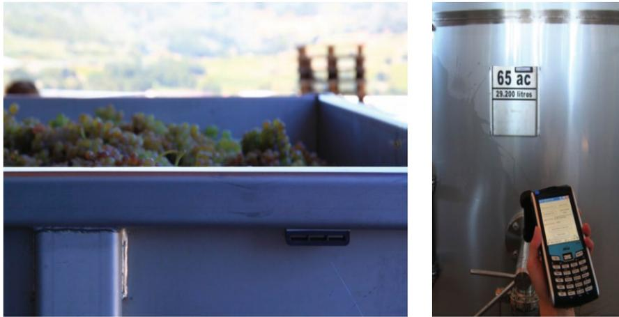
Fig.4. RFID tags attached to containers of grapes [33]
