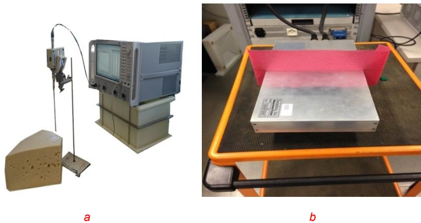
*Fig. 4. Different characterization methods a) dielectric characterization of cheese using a coaxial probe b) characterization of thin sheets of casein in a resonant cavity*
