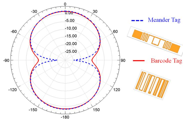
*Fig. 13. Comparison between the simulated directivities of a conventional meander tag and proposed barcode tag design.*
