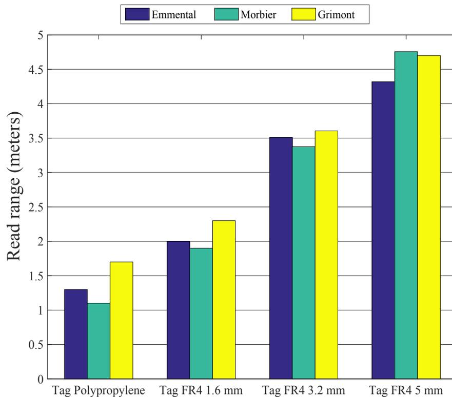
*Fig. 19. Comparison between measured read ranges of different configuration on three types of cheese.*
