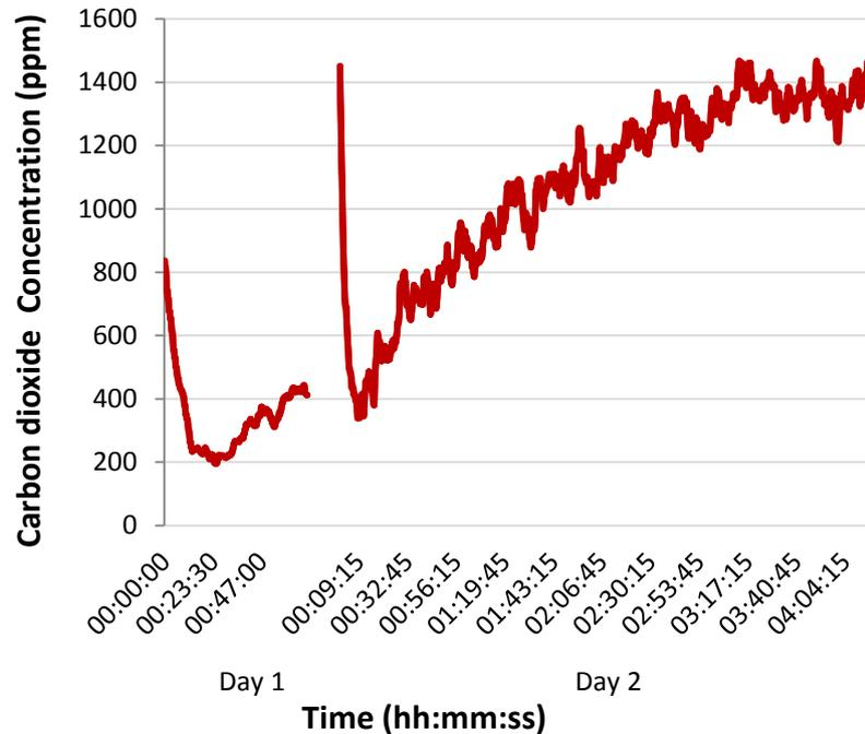
*Fig. 10. Results obtained from the CO<sub>2</sub> sensor over two days in the warm ripening chamber.*
