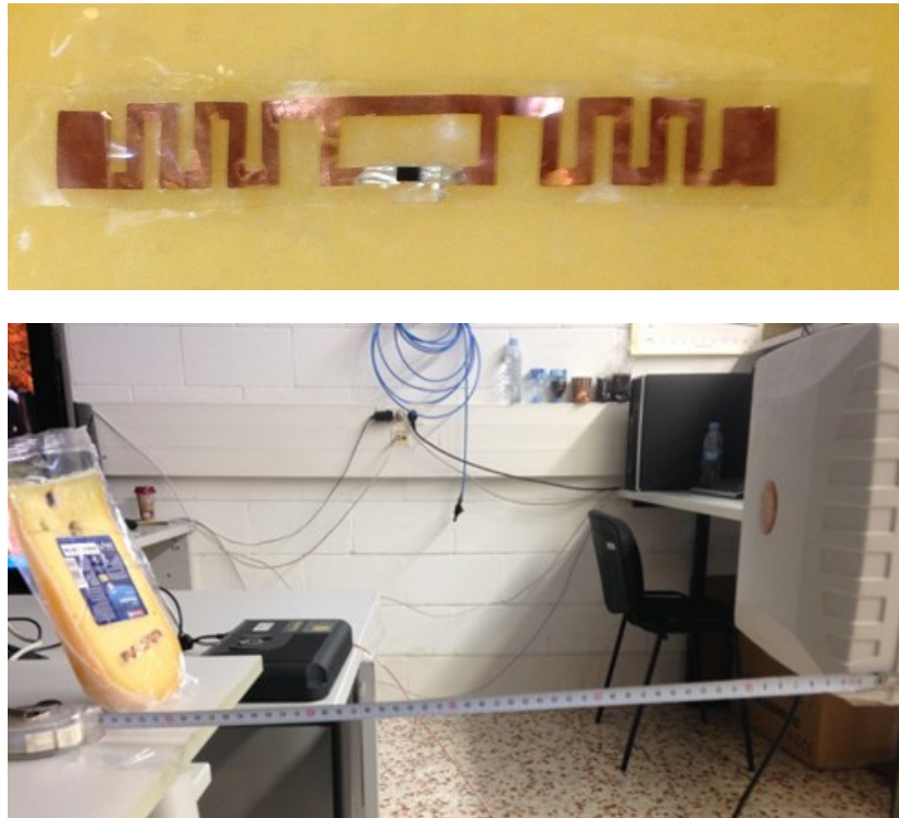
Fig. 23. a) Realized tag prototype on PLA b) Measurement setup
