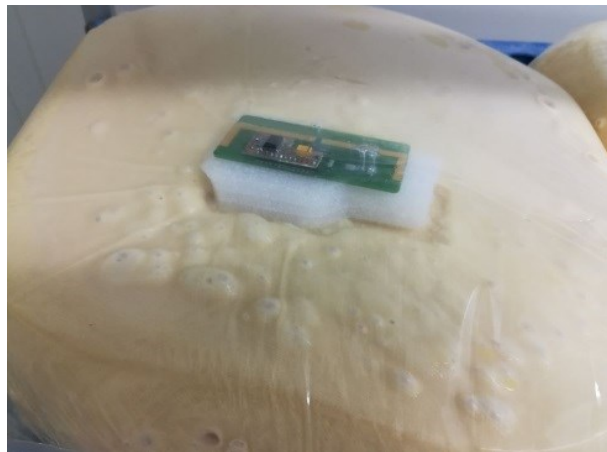
Fig. 16. UHF RFID tag configuration for pressure monitoring inside the cheese package a) cheese package under vacuum with tags on top b) Creation of bubbles in the cheese texture due to gas release which results into an increase of pressure
