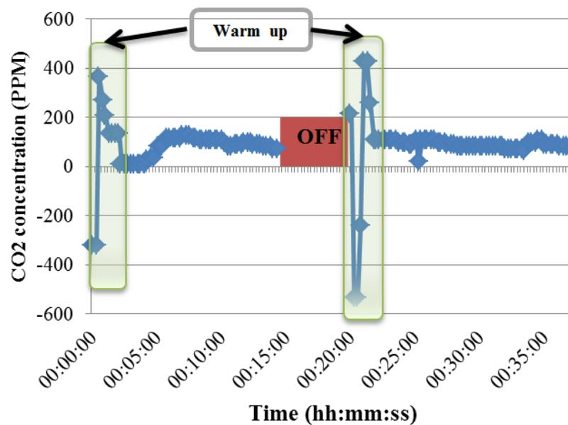
*Fig. 9. Results obtained from CO<sub>2</sub> sensor with a turn off period between measurements*
