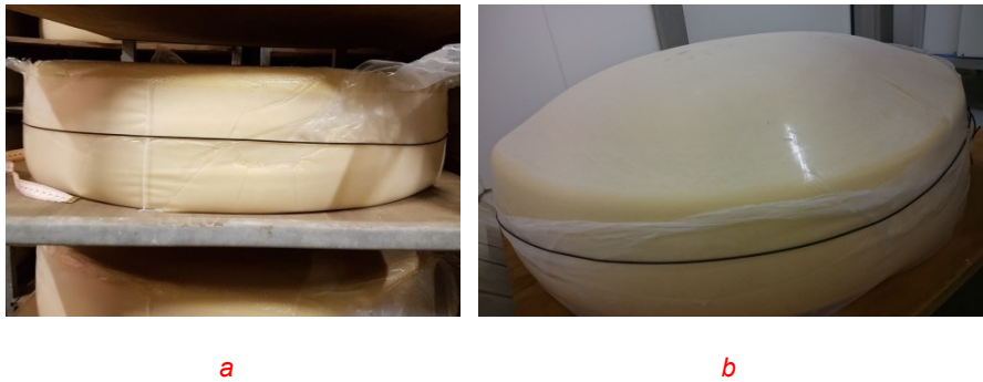
Fig. 11. Stretch resistive sensor installed on Emmental cheese wheel a) start of ripening b) end of ripening
