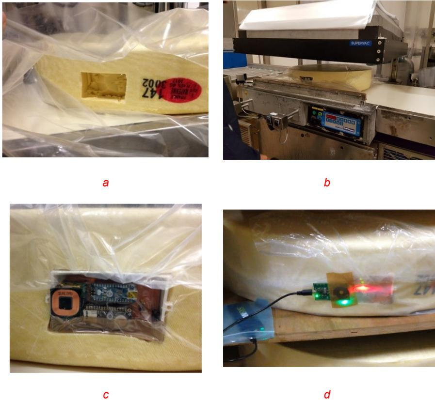
*Fig.8. CO<sub>2</sub> sensor installation a) Removing parts of the curd to install the sensors b) Cheese wheel wrapping c) Sensor integrated in the cheese packaging d) Measurement setup in warm cave where the sensor is powered by inductive coupling.*
