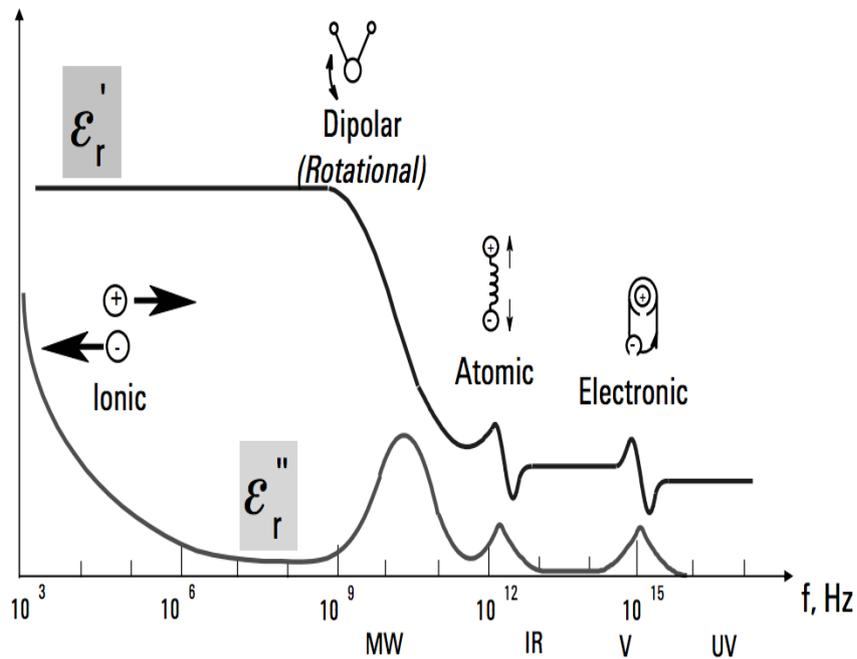
Fig. 4. Typical frequency-regions of the loss mechanisms
