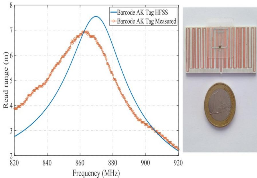
*Fig. 20. Measured read range vs. HFSS simulation of an AK Tag coupled to EAN barcode at the optimum coupling position.*
