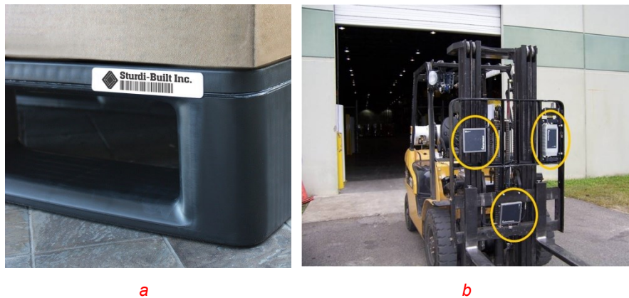
Fig.3. Example of RFID system for supply chain management a) RFID tag on pallet b) Vehicle-mounted readers are placed on forklifts to automatically read and record the data registered in the pallet's RFID tag [16], [17]
