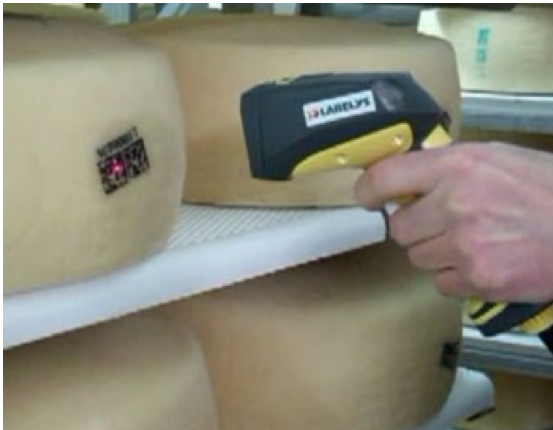
Fig. 2. Cheese traceability system based on Barcodes [3]
