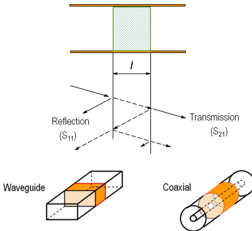
*Fig. 12. Dielectric characterization based on enclosed transmission lines*
