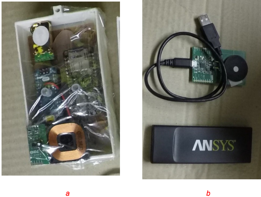
Fig. 7. CO 2 sensor powered by coupling a) Rx coupling module connected to the sensor circuit b) Tx coupling module powered by a USB battery pack
