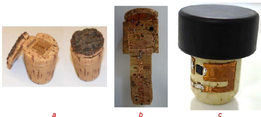
Fig. 5. Different configurations of RFID tags designed on cork a) Meander tag on wine barrel cork b) Meander monopole on wine bottle cork c) compact size tag on regular bottle stoppers [34]
