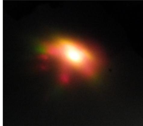
Figure 4.2 Dotted pattern is observed at the output of the ZnSe.
