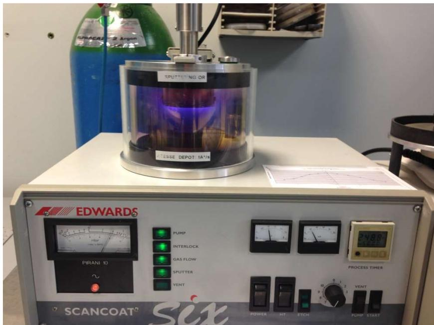
Figure 2-4 Gold metallization setup, Scancoat 6 from Edwards.
