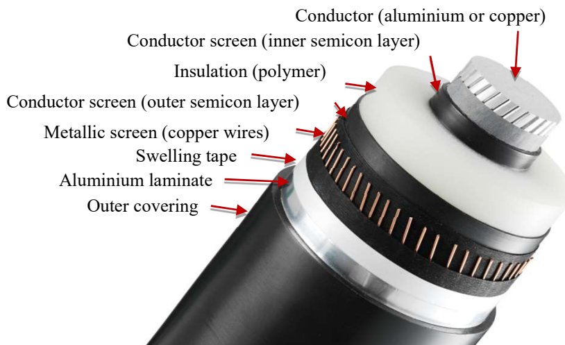
Figure 1-1 Internal layer in a high voltage coaxial cables.
