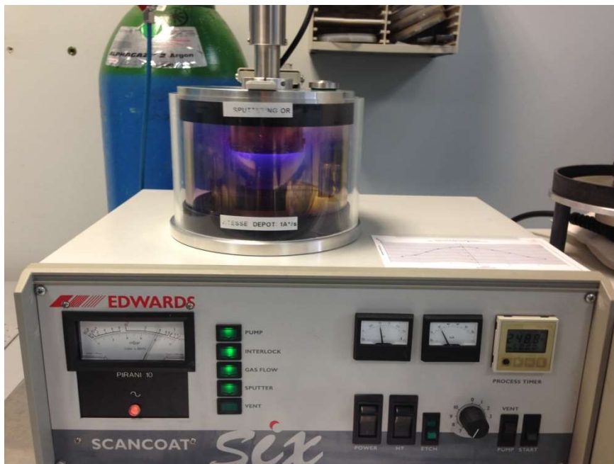
Figure 2-4 Gold metallization setup, Scancoat 6 from Edwards.
