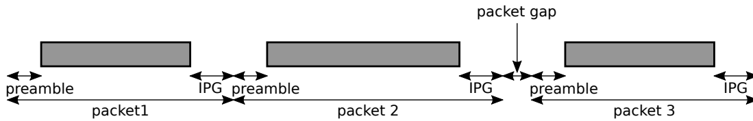
Figure 3.10 – Gaps between consecutive packets on a link when not full
