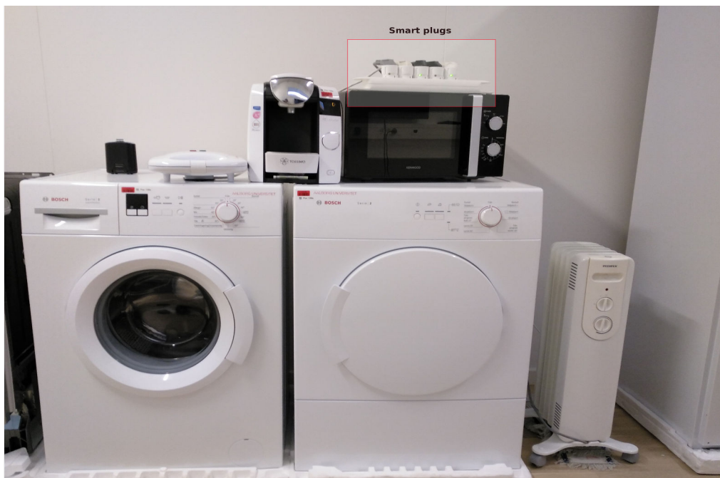
Figure 4.8 – Smart home appliances attached to smart plugs
