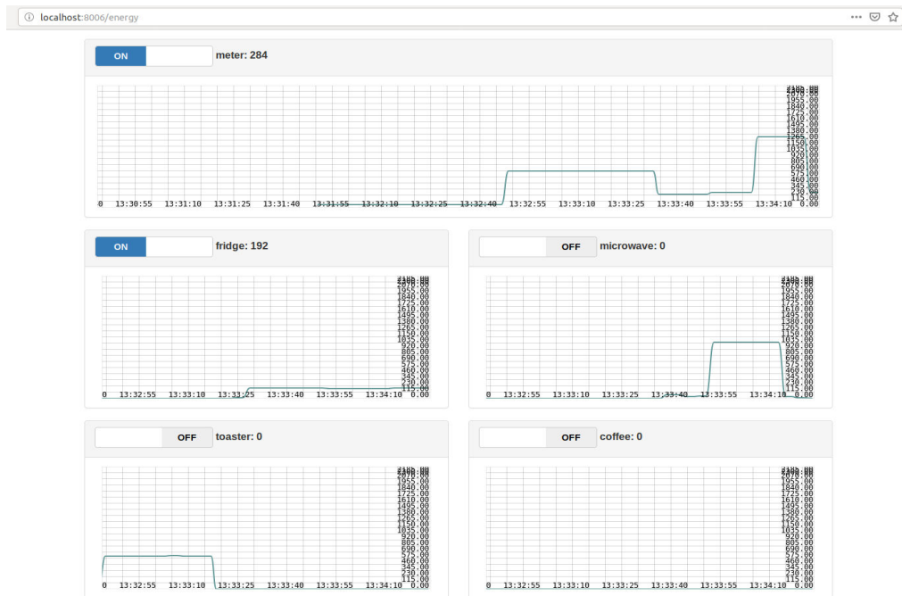
Figure 4.13 – Energy consumption from the smart plugs
