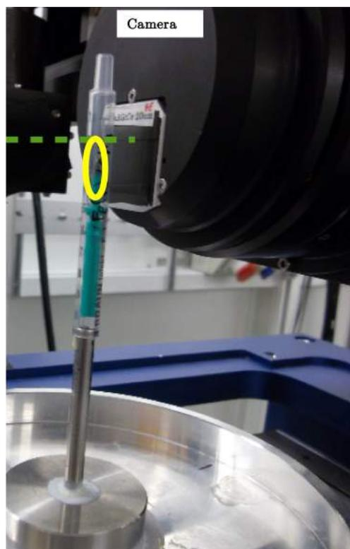
Figure 3.14: Picture of the experimental set-up. Green line corresponds to X-ray beam. Yellow circle corresponds to the sample tip.
