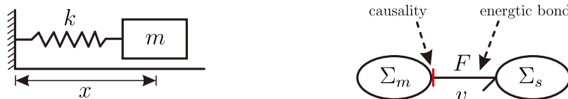
Figure A-1: Example of a mass-spring system (left), and the bond graph representation (right).
