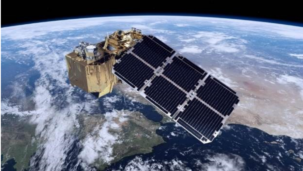
Figure 1.3: The Sentinel-2 satellite.
