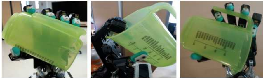
Figure 4.9: Representative grasps on the "measuring cup" show how different grasps may indicate distinct features.
