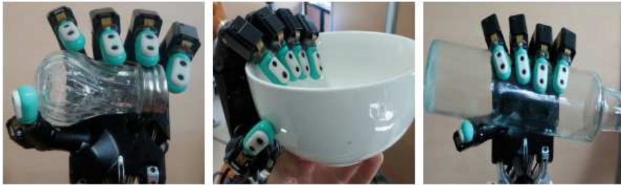
Figure 4.6: Examples of object grasps by the Shadow Hand.
