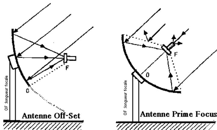
Figure IV-26 : Antenne off-set et prime focus
