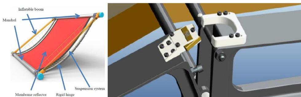
Figure I-5 : Ossature gonflable-rigide (Chang, et al., 2014)
