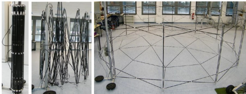
Figure I-16 : Double pantographe (Datashvili-2, et al., 2014)
