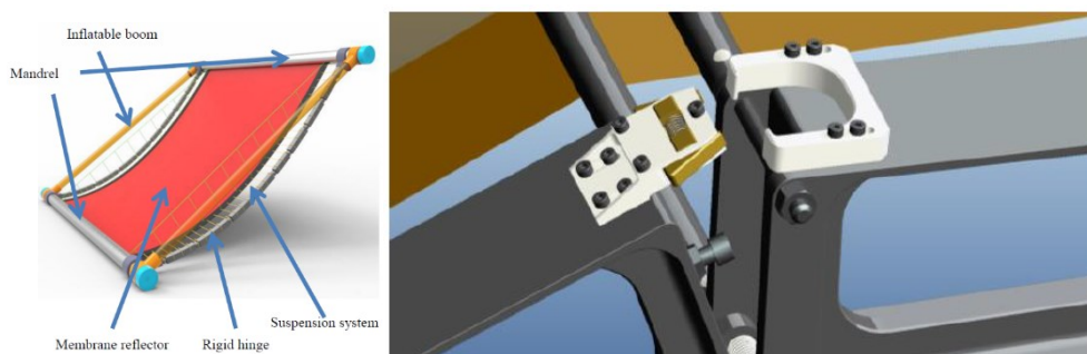
Figure I-5 : Ossature gonflable-rigide (Chang, et al., 2014)
