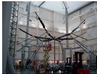
Figure I-9 : Harris mesh reflectors (Mangenot, 2010)
