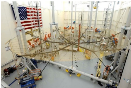
Figure I-9 : Harris mesh reflectors (Mangenot, 2010)
