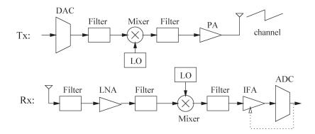
Figure 3.4: Typical transceiver structure
