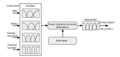
Figure 4.4: Structure of fuzzy logic system
