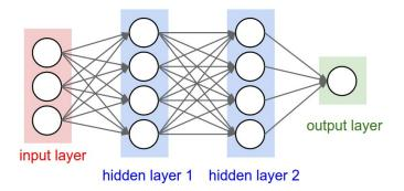
Figure 2.3: Architecture of two hidden layers neural network.
