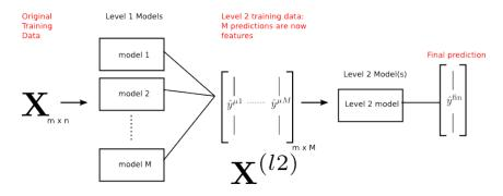
Figure 5.11: Illustration of stacking ensemble machine learning algorithm.
