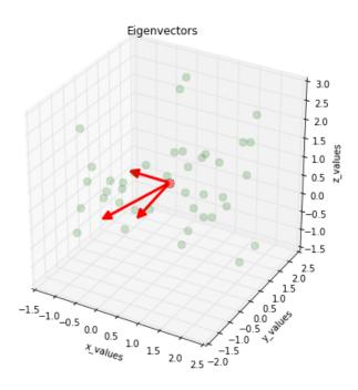
Figure 2.4: Visualization of eigenvectors in Principal component analysis (PCA).
