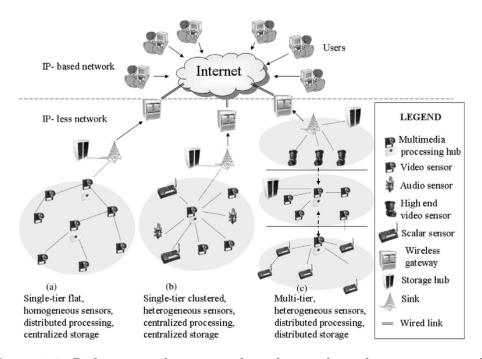
Figure 1.2: Reference architecture of wireless multimedia sensor network.
