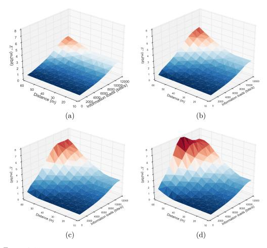
Figure 3.15: 3D plots of effective energy consumption  $E^*$  with multivariate parameter sets ( $\Phi$ , d,  $N_0$ ): (a)  $N_0 = 10$ , (b)  $N_0 = 15$ , (c)  $N_0 = 18$ , (d)  $N_0 = 20$ .
