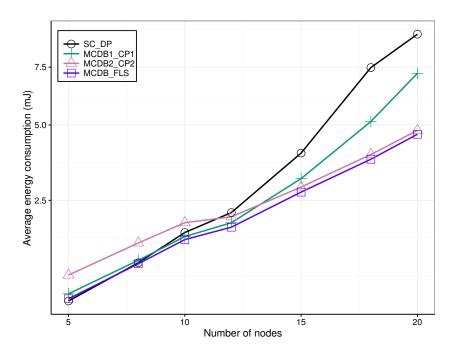
Figure 4.13: Average effective energy consumption of different sensor nodes
