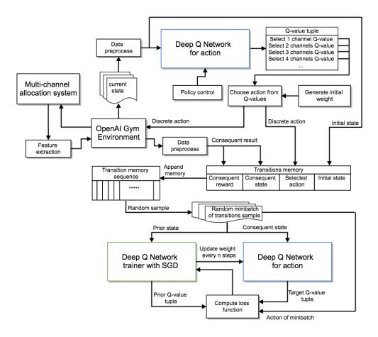
Figure 5.1: Reinforcement learning of multi-channel allocation with deep Qnetwork (DQMC)
