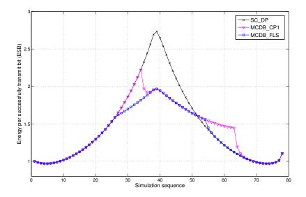
Figure 4.11: Instant effective energy consumption of different schemes
