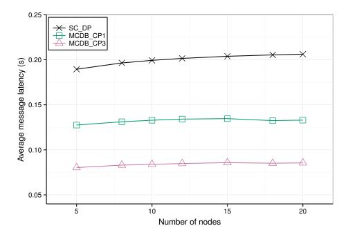
Figure 4.10: End-to-end delay of different sensor nodes
