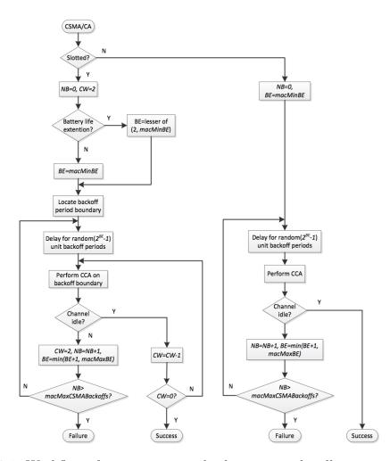
Figure 3.1: Workflow of carrier sense multiple access with collision avoidance algorithm.
