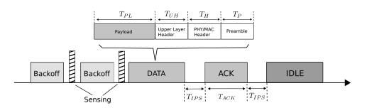
Figure 4.3: IEEE 802.15.4 frame exchange sequence
