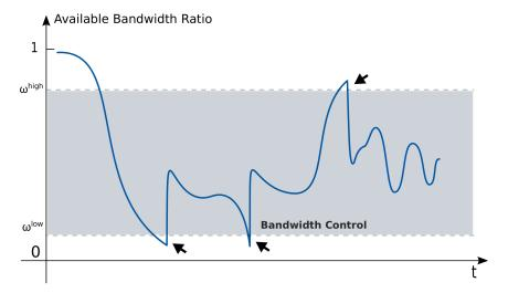
Figure 4.1: Estimation-based adaption of available bandwidth ratio
