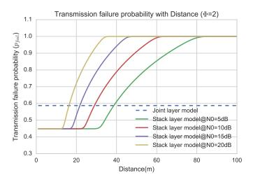
Figure 3.7: Transmission failure probability with distance
