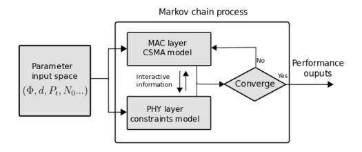
Figure 3.2: stack cross-layer model structure
