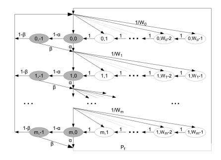
Figure 3.3: Markov chain transition states diagram for CSMA/CA algorithm in IEEE 802.15.4
