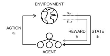
Figure 2.5: Interaction visualization of reinforcement learning.
