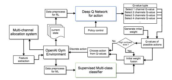
Figure 5.9: DQMC with initial weight fusion using multi-class classifier
