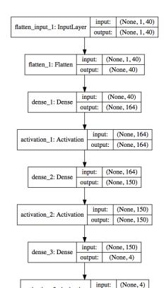
Figure 5.2: Structure of neural network layers
