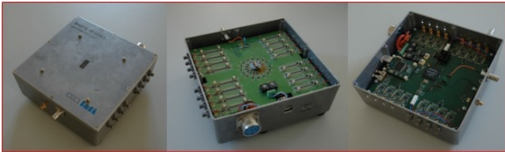
Figure 2.1: Detector setup developed in CEA-LETI: shield aluminium box (left), analog read-out circuit (center) and digital circuit (right).
