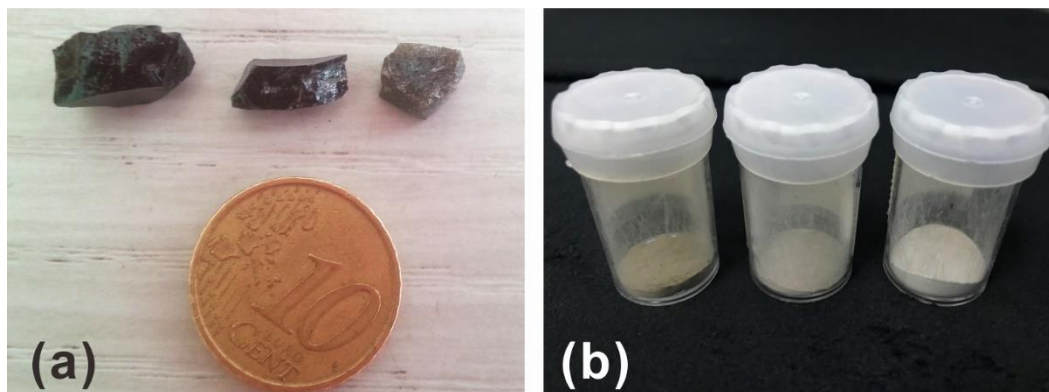
Fig. 3.1 (a) Experimental starting material: dry glasses; (b) the powder of dry glass
