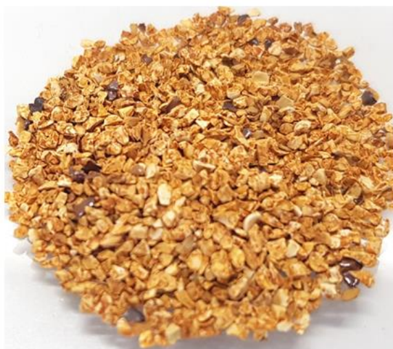
Dried Fe-HZSM-5 After wet impregnation
