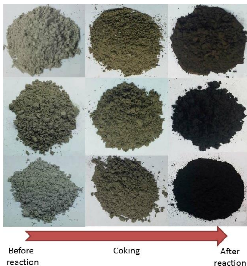
Figure 1.21: Change in physical aspect of catalyst before and after catalytic pyrolysis (Adapted from Rostami et al. , 2015))
