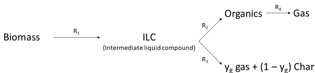
Figure 1.14: Broido-Shafizadeh model for biomass pyrolysis (Shafizadeh, 1982)
