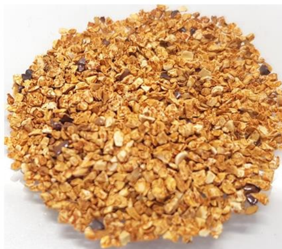
Dried Fe-HZSM-5 After wet impregnation
