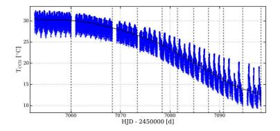
Figure B.4: Changing on-board CCD temperature with respect to time for the setup 6 data of  $\zeta$  Ori of the Orion II campaign of BLb. The long-term behaviour is approximated by a local linear regression filter, which constructs a total of ten different time windows using both a temperature threshold of 2 °C and a data gap criterion of 0.5 d. The correlation for the first window is shown in Fig. B.5.
