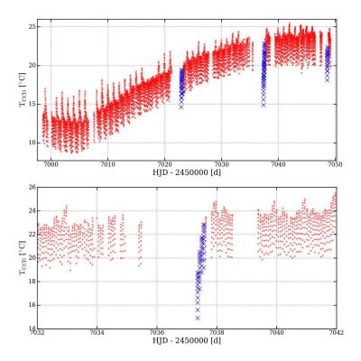
Figure B.2: Top: Varying on-board temperature, measured at the CCD, is indicated in red for the setup 5 file of  $\zeta$  Ori of BHr during the Orion II campaign. The orbits having a different long-term behaviour are rejected and indicated by blue crosses, which mostly happens after a significant data gap. *Bottom*: Zoom of the top panel around the second gap region at HJD=2457037.
