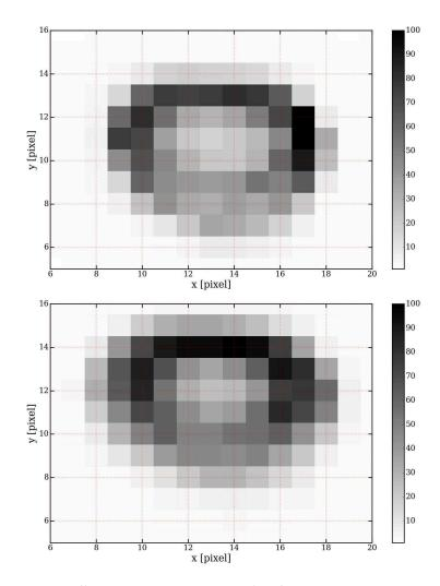
Figure B.3: Two different observations of  $\zeta$  Ori during the setup 7 Orion II campaign for BHr. The top image was taken with an on-board temperature of 21.49 °C, while the bottom image has a  $T_{\rm CCD}$  of 17.57 °C. The normalized counts per pixel is represented by the grayscale. Differences are seen in the width, the sharpness, and the location of the maximum of the non-Gaussian PSF.
