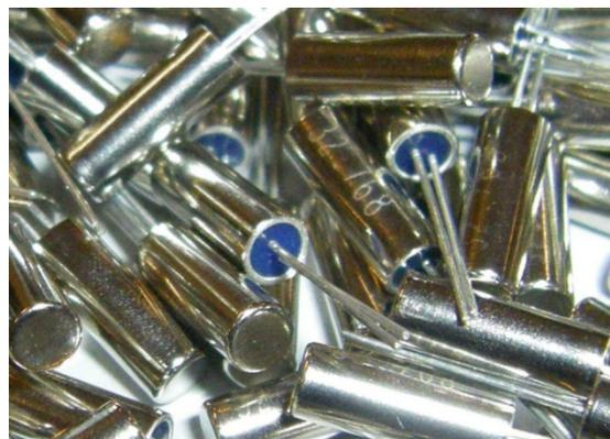
**Figure 3-2: Quartz tuning fork with a capsule cover**
