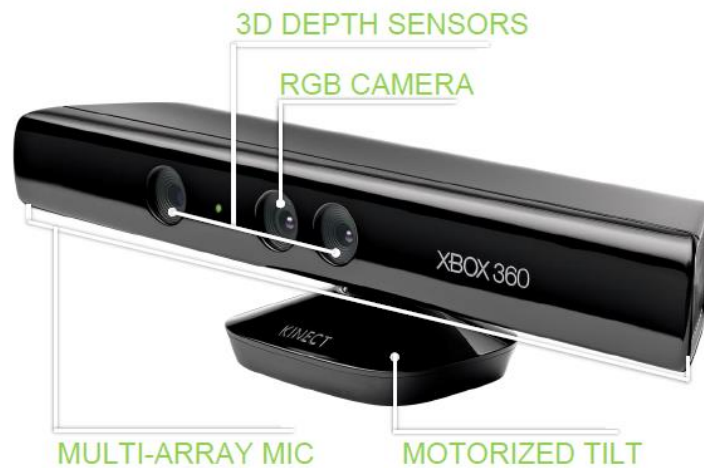
Figure 15. Kinect camera and its components (source: reference 94)
