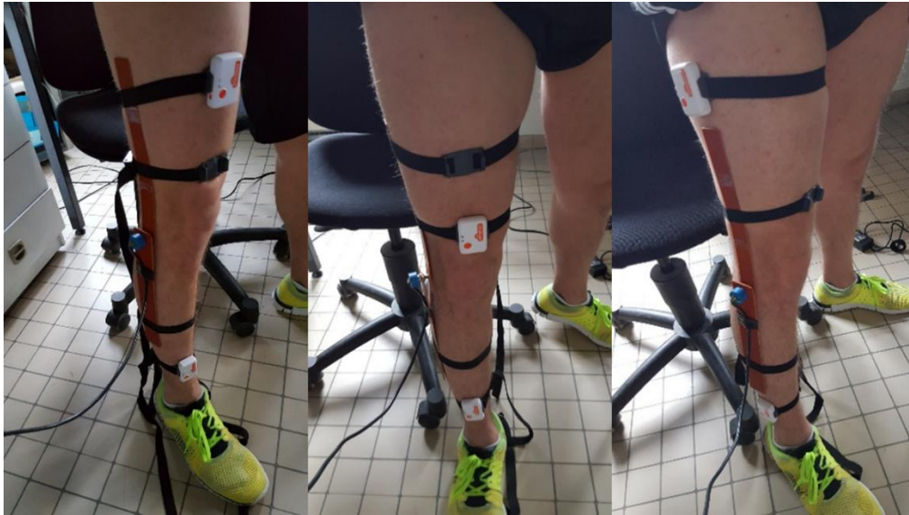
Figure 53. Tested sensor positions (Left: sensor on the thigh directly; Middle: sensor above the kneecap; Right: sensor in the sagittal plane)
