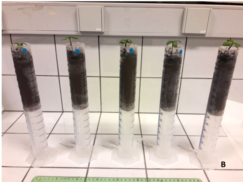
Figure S3: Soil column experiments. (A) Soil column design, before introducing sunflower seeds; (B) After 5 days growth, sunflowers with magnNPs-Cu treatment.
