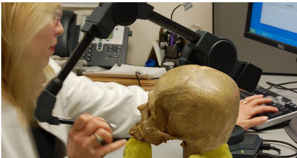
Figure 39 : Microscribe en situation d'acquisition (osteoware.si.edu).
