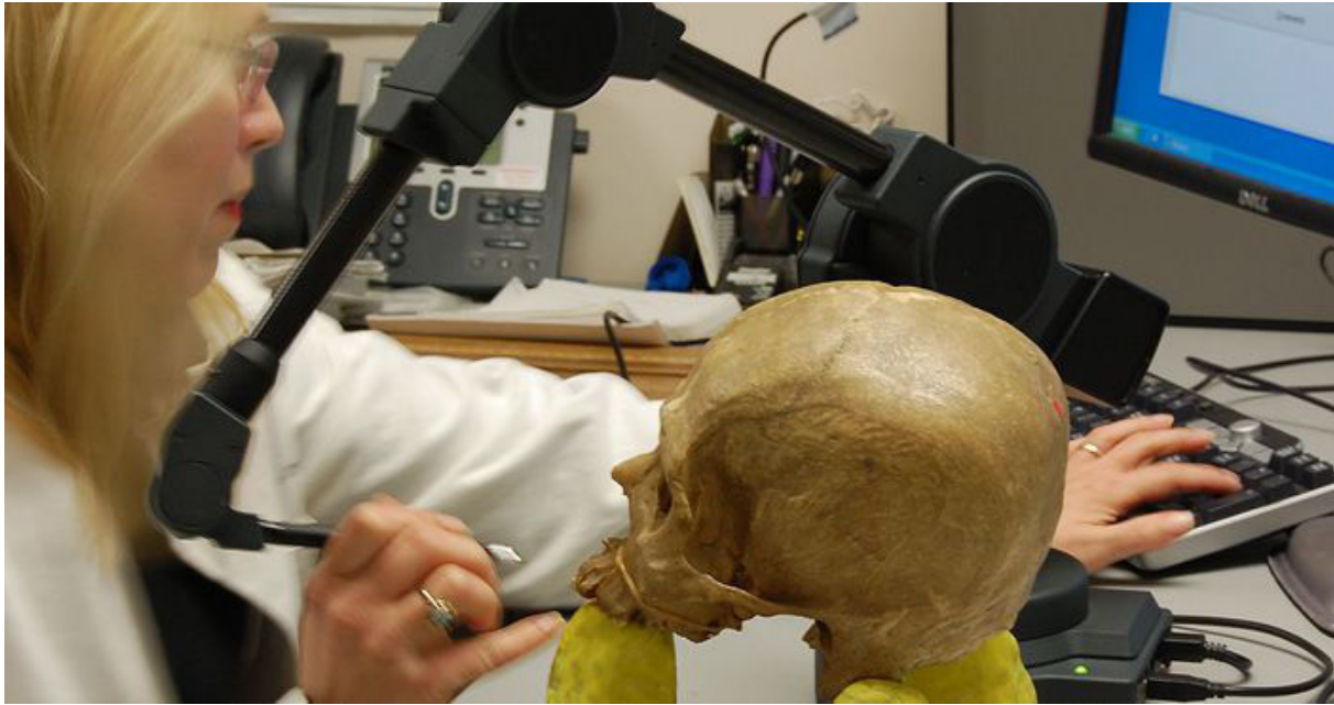
Figure 39 : Microscribe en situation d'acquisition (osteoware.si.edu).
