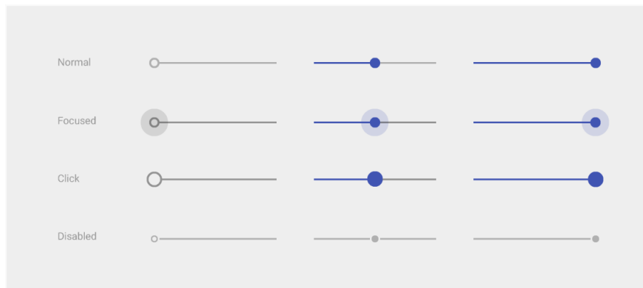
Figure 2-9: Google's design guidelines for different states of a graphical slider. When unused (normal), the slider presents a small sized knob. When being used (focused and click), the knob increases its size. When the slider is unavailable (disabled), the knob becomes very small.
