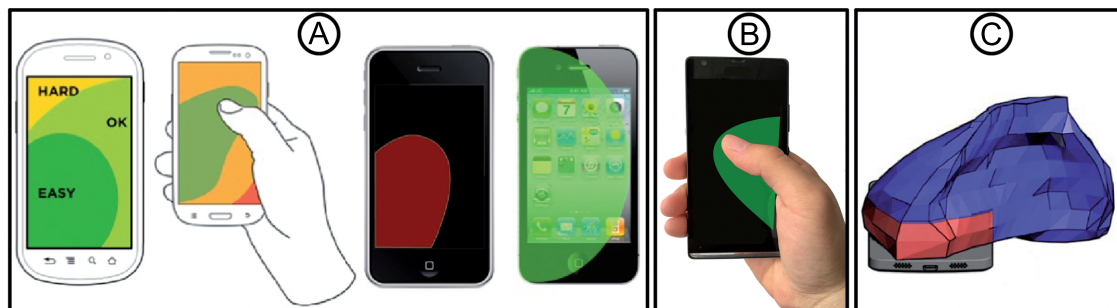
Figure 2-5: Functional area of the thumb according to: (A) heuristic models, and (B) a predictive model. (C) Functional workspace of the thumb. Figure from [31, 38, 71, 182, 62]
