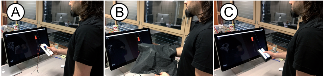
Figure 5-18: A participant performing the experiment under different conditions: (A) Tangible slider with visual feedback. (B) Tangible slider with no visual feedback. (C) Graphical slider with visual feedback.
