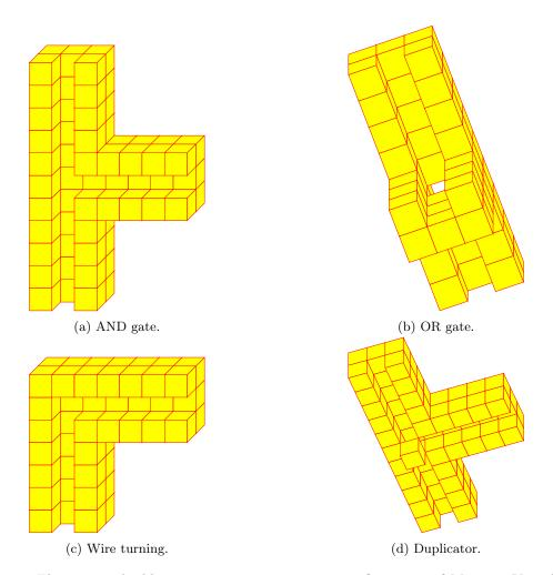
Figure 4.6: Elements to build any monotone circuit on a configuration of Majority-Vote Cellular Automata.
