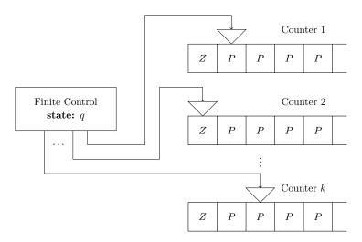
Figure 4.1: Scheme of a k-counter machine.
