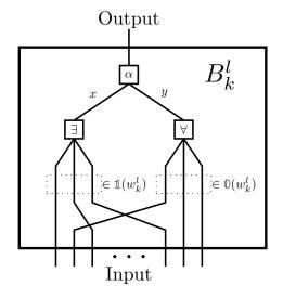
(a) Neighborhood matcher  $B_k^l$ . Notations  $\mathbb{O}(w)$  and  $\mathbb{1}(w)$  stand for the set of all indexes i s.t.  $w_i = 0$  and  $w_i = 1$  respectively. This block triggers a 0 on the output wire exactly when the input is  $w_k^l$ .
