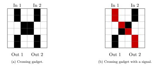
Figure 5.4: Crossing signal in Moore neighborhood. If the cell in In 1 (2) is in state  $\blacksquare$ , then after five iterations the cell in Out 2 (1) change to state  $\blacksquare$  (as seen on Figure 5.4b).
