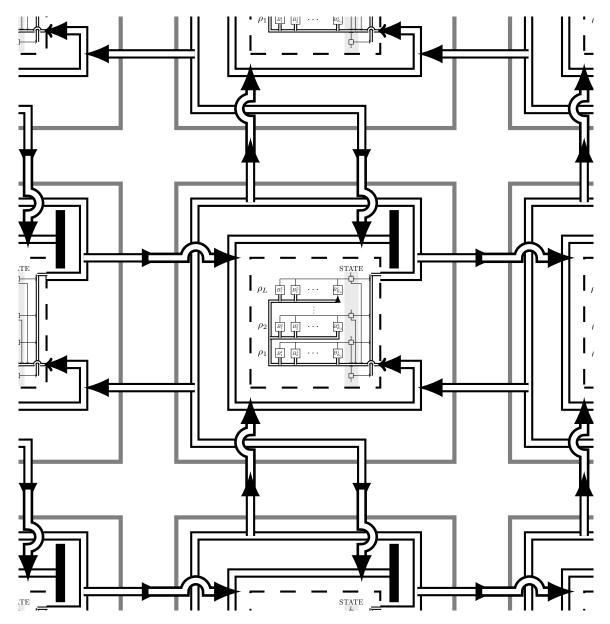
Figure 5.2: The dashed block in the middle is a macro-cell, as in figure 5.1b. The fat arrows exchange the state of each macro-cell with its neighbors.
