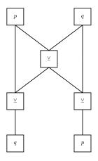
Figure 4.4: Building a crossing gate from XOR gates.
