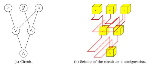
Figure 4.7: Example of a simulation of a circuit by the Majority-Vote Cellular Automata.
