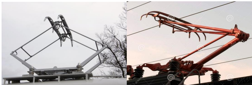
Figure 18. Old pantograph (left) vs new pantograph (right)
