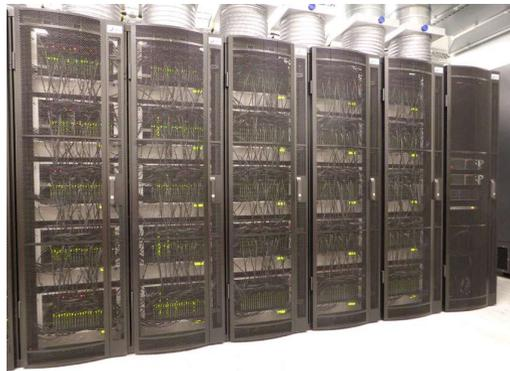
Figure 15: The 500 000 cores SpiNNaker Human Brain platform. Extracted from [70].
