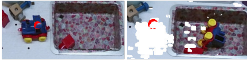
Figure 5.4: Visualisation of the change detector. The right picture represents a part of a scene before a push and the left picture after a push. The red dot on both pictures represents the target of the push primitive which is here the upper part of the blue toy. This target corresponds to the center of a supervoxel. The white areas represent the parts detected as different between both images.
