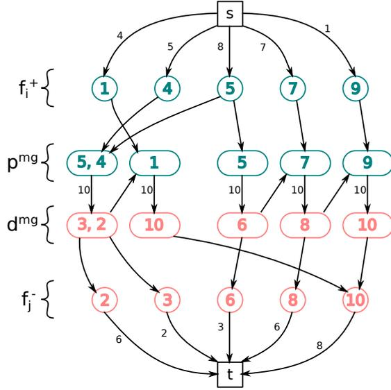
Figure 12: Resulting flow graph of the routes in the solution of Figure 10 assuming vehicles with capacity  $C = 10$ . The labels on the arcs are the capacities of each arc (infinite capacities are omitted).
