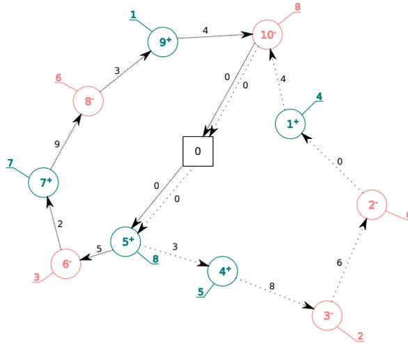
Figure 10: Example of feasible solution for the graph depicted in Figure 9 assuming a capacity  $C = 10$  and using 2 vehicles. Each arc has a label reporting the load of the vehicle after visiting a node. Node 5 and node 10 are visited by both vehicles splitting their demands.
