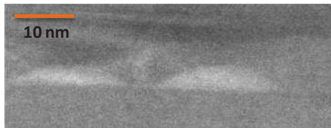
Figure II-12. Cross-sectional HAADF-STEM image of the GaN QD / Al_{0.6}Ga_{0.4}N structure (sample E).
