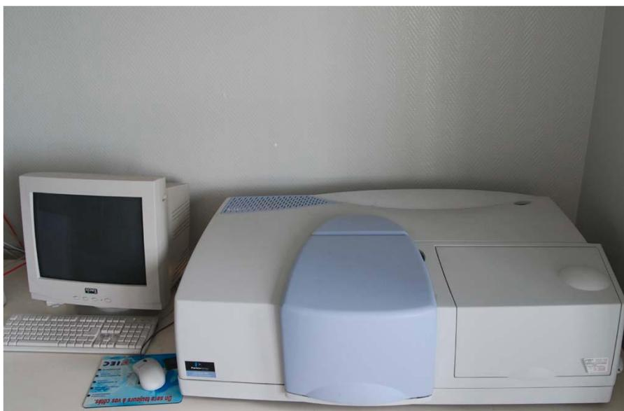
Figure 20 : Spectrometre Perkin Elmer Lambda
