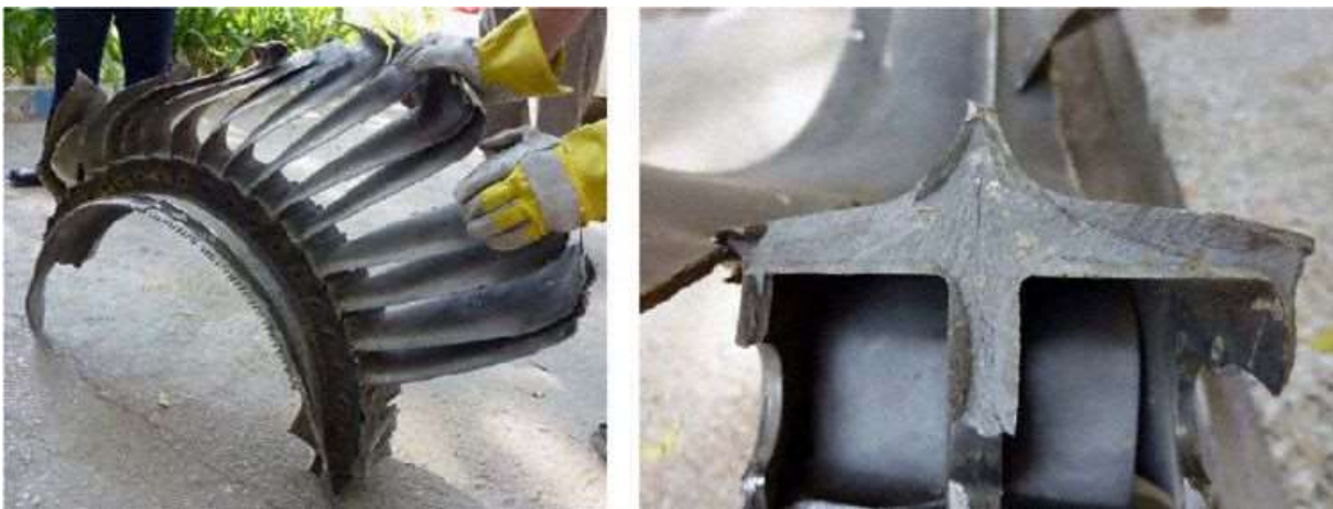
Figure 1-4: Photographs of the recovered low pressure compressor 2 nd stage disk (Photo: SIB).
