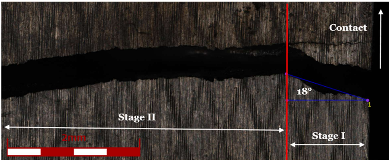
Figure 4-5: Angle of the crack initiation and profile of the crack propagation for the specimen under the contact of the cylinder pad with radius R=70\text{mm} .
