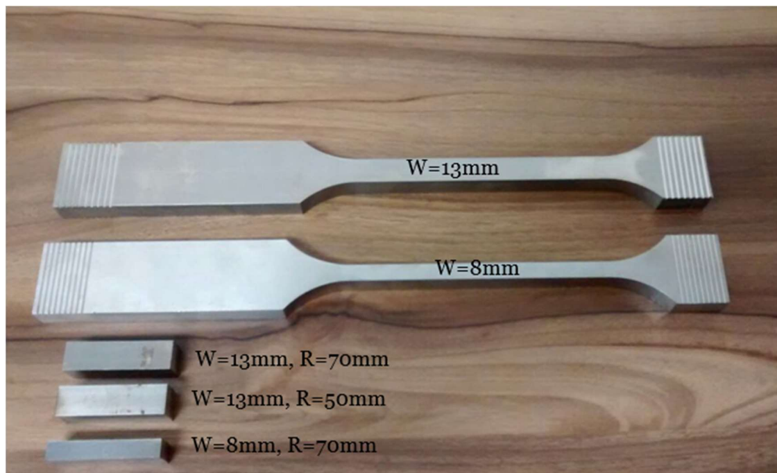
Figure 3-9: Photograph of fretting fatigue specimens and pads.
