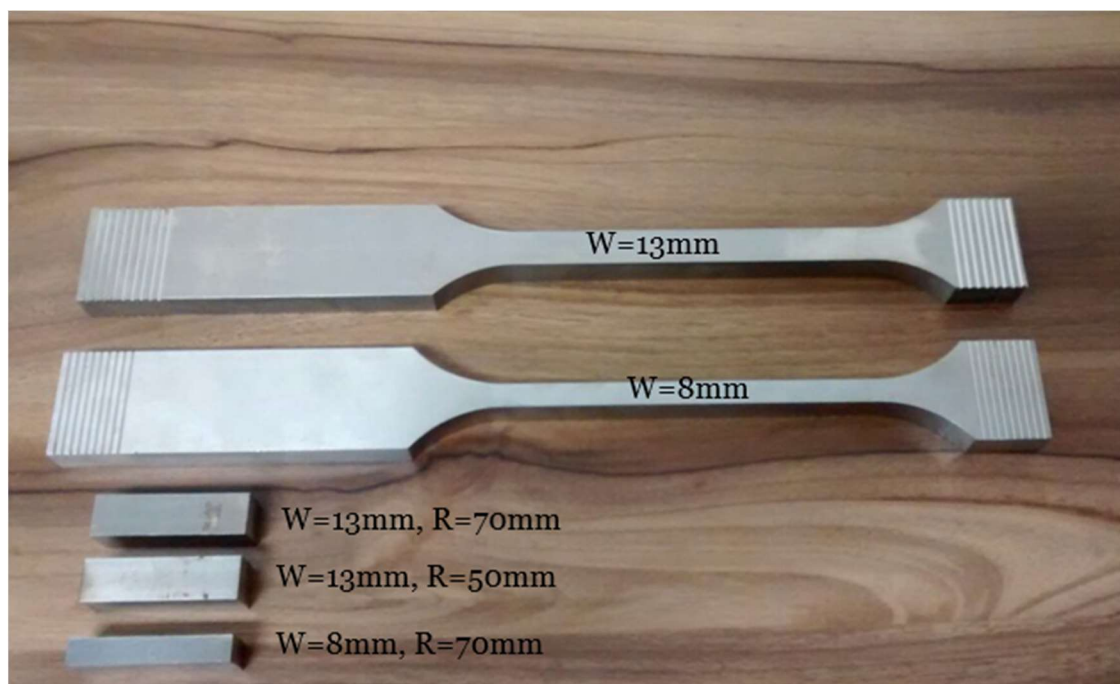
Figure 3-9: Photograph of fretting fatigue specimens and pads.
