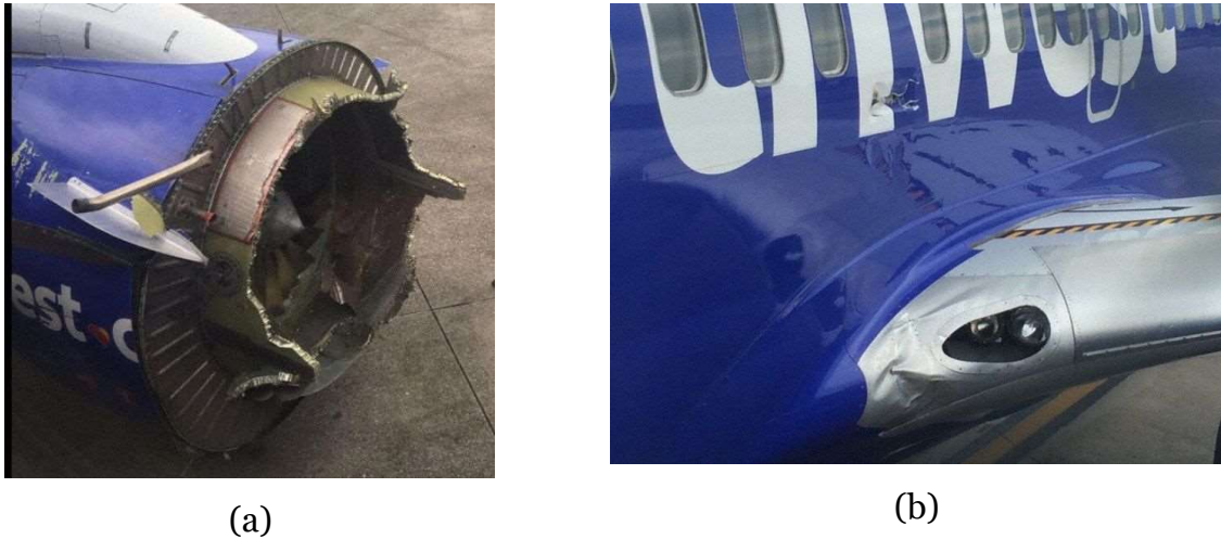
Figure 1-3: Photographs of an aircraft (a) engine and (b) fuselage damage in a Southwest Airline's Boeing 737-700 in August, 27 th 2016 near Pensacola (Photo: Peter Lemme).
