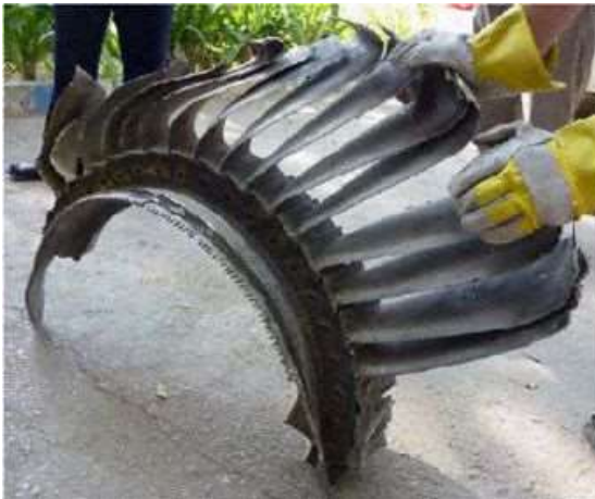
Figure 1-4: Photographs of the recovered low pressure compressor 2 nd stage disk (Photo: SIB).
