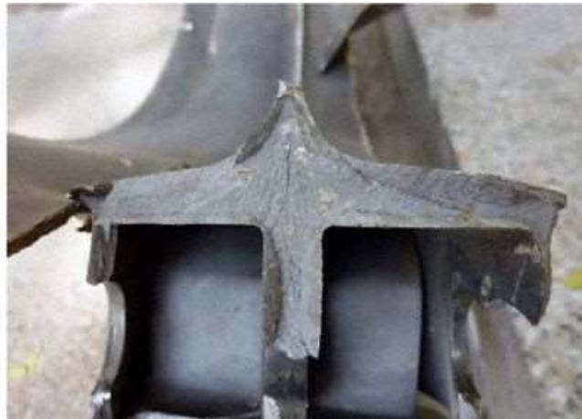
Figure 1-4: Photographs of the recovered low pressure compressor 2 nd stage disk (Photo: SIB).
