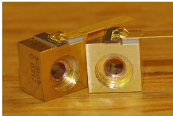
Figure II-19: Optical view of the final micro assembled device on a C-mount heat sink.
