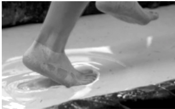
Figure 4.2: Snapshot of a person running on top of a pool filled with a dense suspension of cornstarch and water. The fluid can temporarily hold up the person's weight like a solid, sustaining stresses orders of magnitude beyond the capabilities of the suspending Newtonian liquid (here water) (From [6]).
