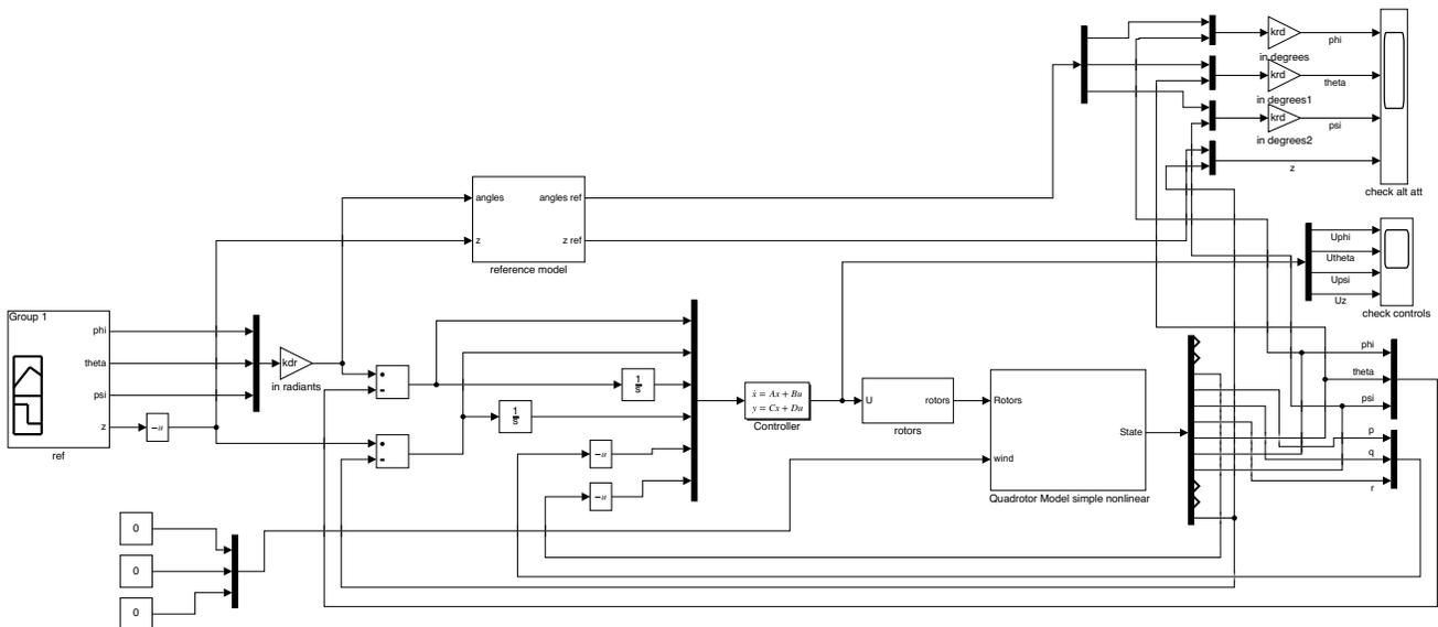
Figure C.7: Closed-loop model in Simulink to test the structured-PID controller.
