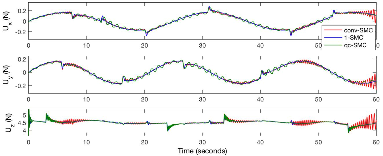
Figure 5.13:  $x$ ,  $y$ ,  $z$  controls using the designed SMCs.
