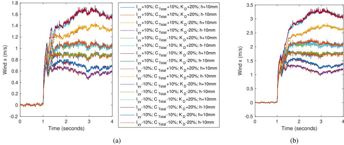
Figure 5.4: Step responses for fusion algorithm to 1 m/s wind speed in (a), to 2 m/s in (b)
