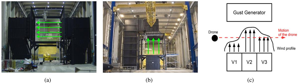
Figure 1.4: Images of the lateral wind gust generator (a), vertical wind gust generator (b) in the B20 lab; and of the produced wind profile over the passage of the drone (c).
