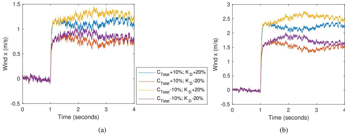
Figure 5.5: Step responses for algorithm-lin to 1 m/s wind speed in (a), to 2 m/s in (b).
