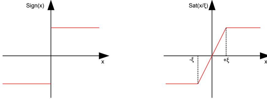
Figure 3.1: Approximation of sign using linear saturation function.
