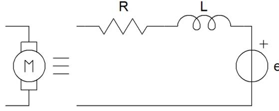
Figure 2.2: Rotor model
