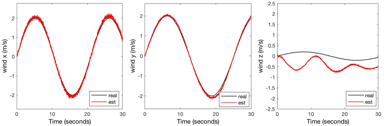
Figure 5.6: Wind estimation using full nonlinear quadrotor model.
