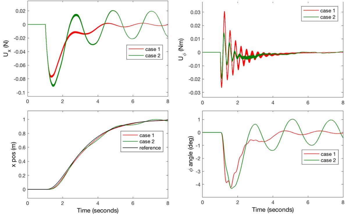
Figure 5.7: Influence of  $\alpha_i$  parameter of qc-SMC for  $x$  and  $\theta$  quadrotor dynamics.
