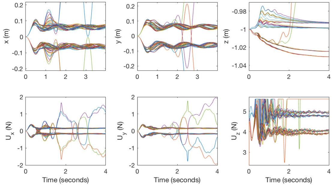
Figure 5.29: Positions ( $x, y, z$ ) and their respective qc-SMC inputs considering wind step estimates, full quadrotor model influenced by coefficients uncertainty and combinations of wind speed steps
