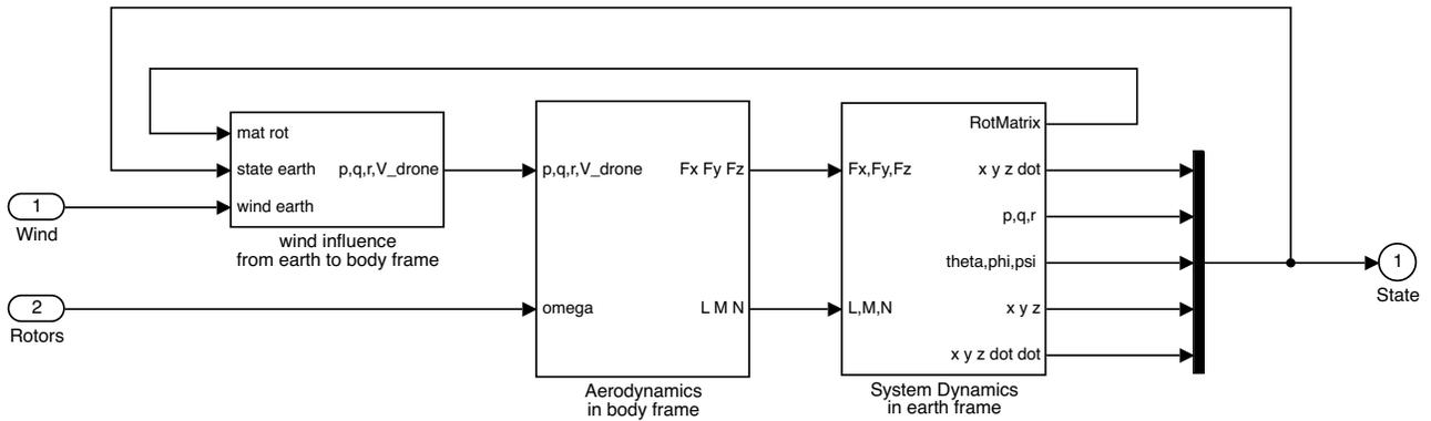
Figure D.3: Second layer of the quadrotor model.
