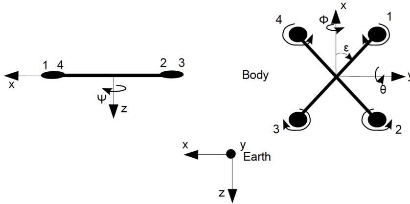
Figure 2.1: Quadrotor configuration with Earth and Body frames.
