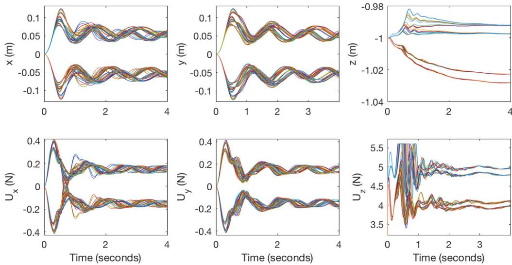
Figure 5.22: Positions ( $x, y, z$ ) and their respective qc-SMC inputs considering fixed  $D_i$ , quadrotor model influenced by coefficients uncertainty, and combinations of wind speed steps with reduced amplitude.
