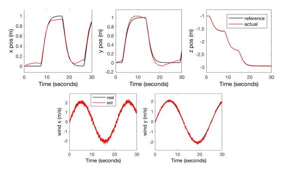
Figure 5.30: Positions (x, y, z) and wind estimates, using qc-SMC inputs considering wind estimates, full quadrotor model and tuned smaller values of  $\rho_i$ .
