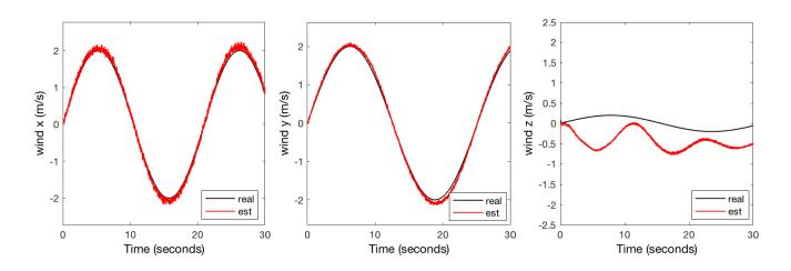
Figure 5.6: Wind estimation using full nonlinear quadrotor model.
