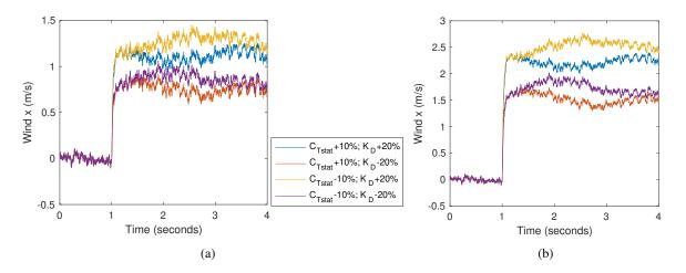
Figure 5.5: Step responses for algorithm-lin to 1 m/s wind speed in (a), to 2 m/s in (b).
