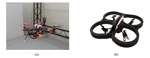
Figure 1.2: Images of the: X4-MaG drone (a); Parrot Ar.Drone 2.0 (b)
