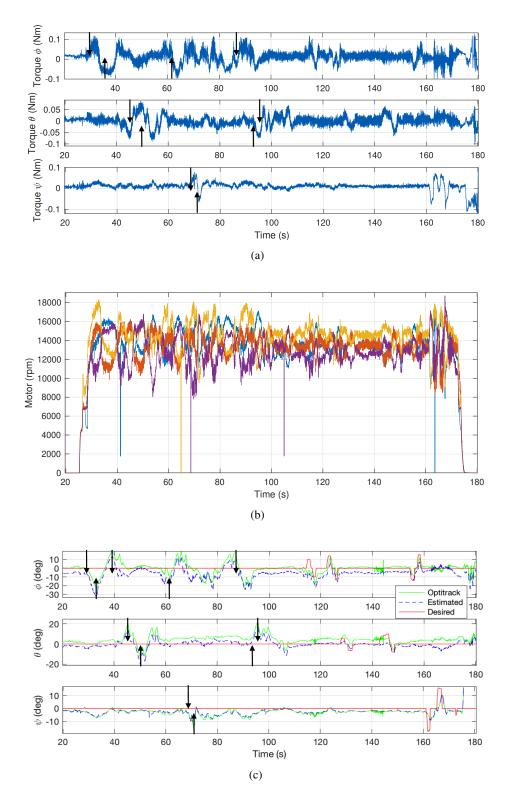
Figure 5.34: Exp 1 using qc-SMC: Computed torques (a), motor velocities (b), desired and actual angles (c).
