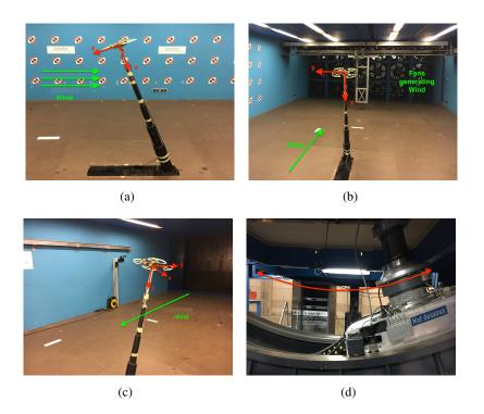
Figure 1.5: Images of the L2 wind tunnel in lateral view (a), frontal view (b), posterior view (c); and of the mechanism that allows the stick to move circularly (d).
