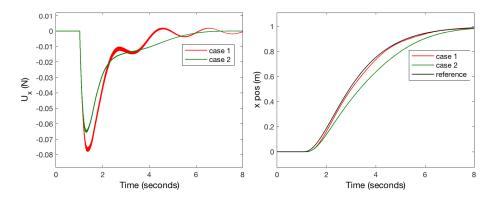
Figure 5.9: Influence of  $\rho_i$  parameter of qc-SMC for x quadrotor dynamics.
