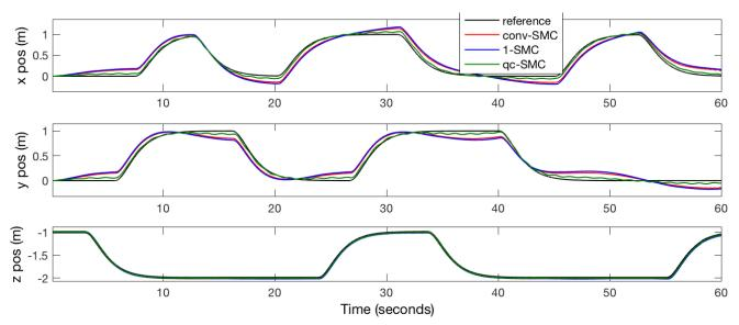
Figure 5.12: x, y, z positions using the designed SMCs.
