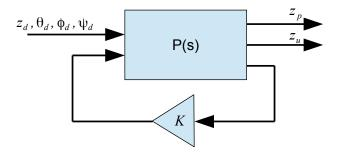
Figure C.4: Standard form for  $H_{\infty}$  design.
