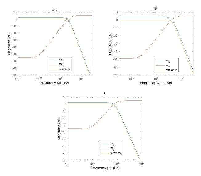
Figure C.3: Weighting functions of reference model.
