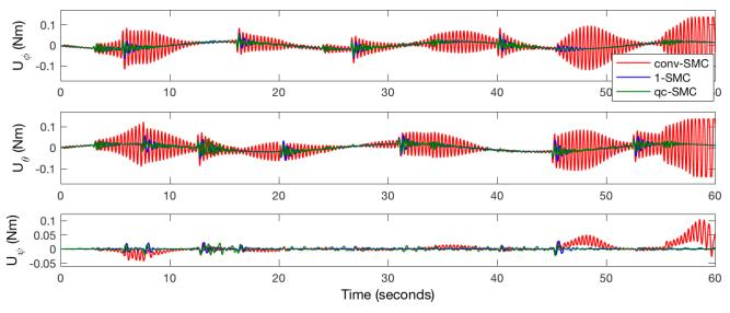
Figure 5.17:  $\phi$ ,  $\theta$ ,  $\psi$  sliding surfaces of the designed SMCs.
