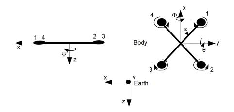
Figure 2.1: Quadrotor configuration with Earth and Body frames.
