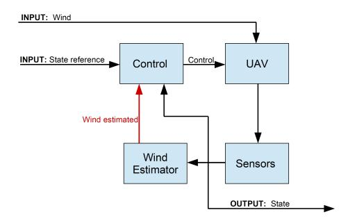
Figure 3.3: Control scheme having as input the wind estimates.
