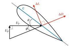
Figure A.6: Forces and wind speed acting on blade section.
