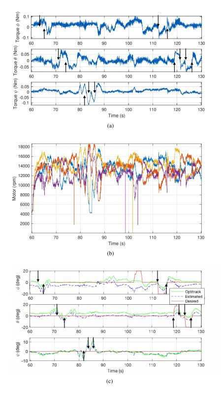
Figure 5.35: Exp 2 using qc-SMC: Computed torques (a), motor velocities (b), desired and actual angles (c).
