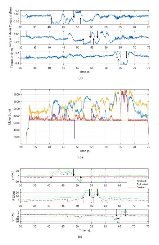
Figure 5.33: PID controller: Computed torques (a), motor velocities (b), desired and actual angles (c).
