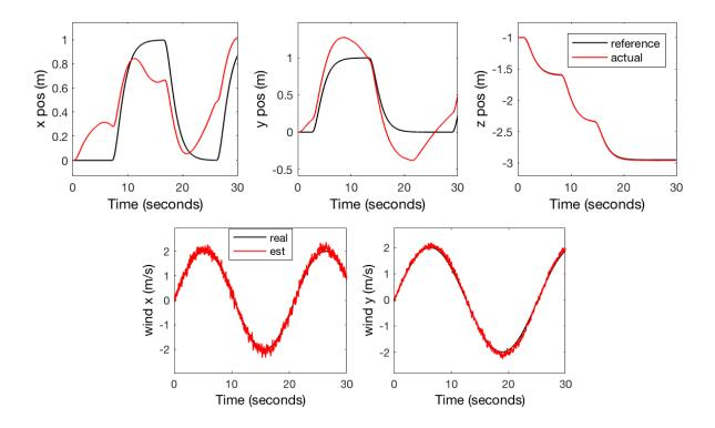
Figure 5.31: Positions (x, y, z) and wind estimates, using qc-SMC inputs considering wind estimates, full quadrotor model and higher values of  $\rho_i$ .
