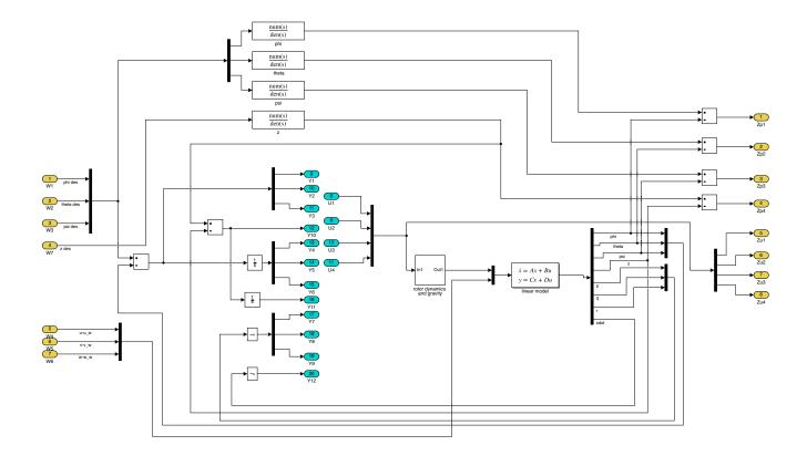
Figure C.6:  $H_{\infty}$  design in Simulink.
