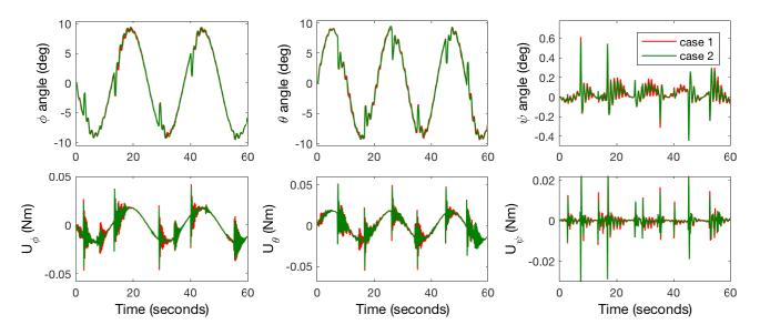
Figure 5.28: Quadrotor angles: Comparison between constant gain  $D_i$  and wind estimates as input to qc-SMC.
