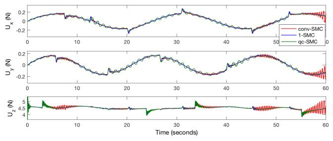
Figure 5.13: *x*, *y*, *z* controls using the designed SMCs.
