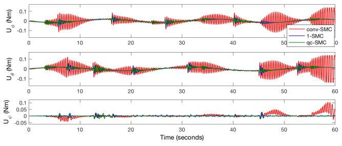
Figure 5.15:  $\phi$ ,  $\theta$ ,  $\psi$  controls using the designed SMCs.
