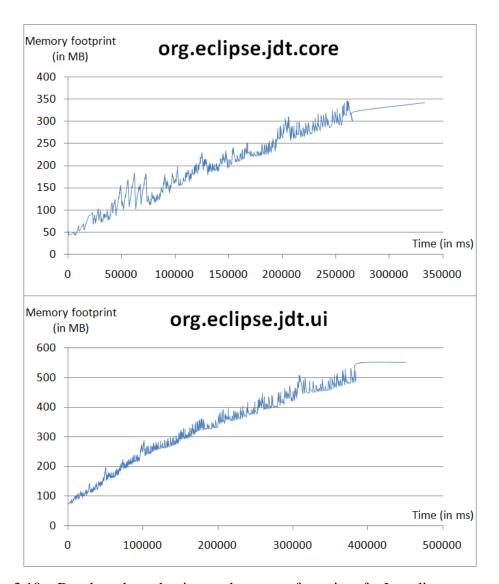
Figure 3.19 – Benchmark on the time and memory footprint of a Java discovery process.
