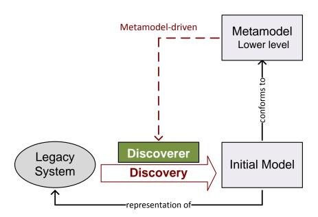
Figure 3.2 – General principle of Model Discovery.
