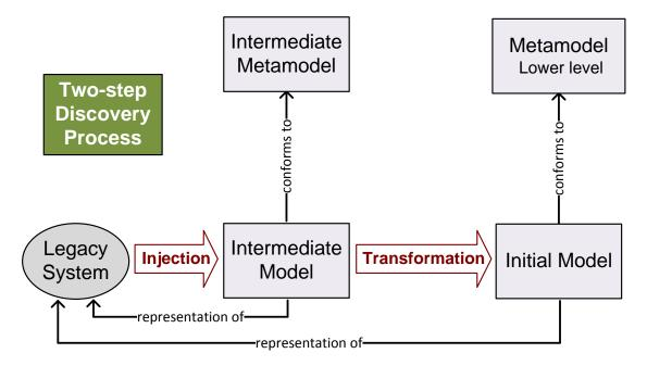
Figure 3.3 – Two-step approach for Model Discovery.
