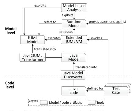
Figure 3.21 – Overall architecture of the fREX framework.
