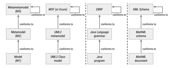
Figure 2.2 – The three-level Modeling stack and similar structuring in the EBNF & XML technical spaces.
