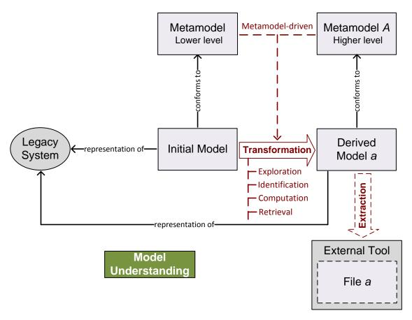
Figure 3.4 – General principle of Model Understanding.
