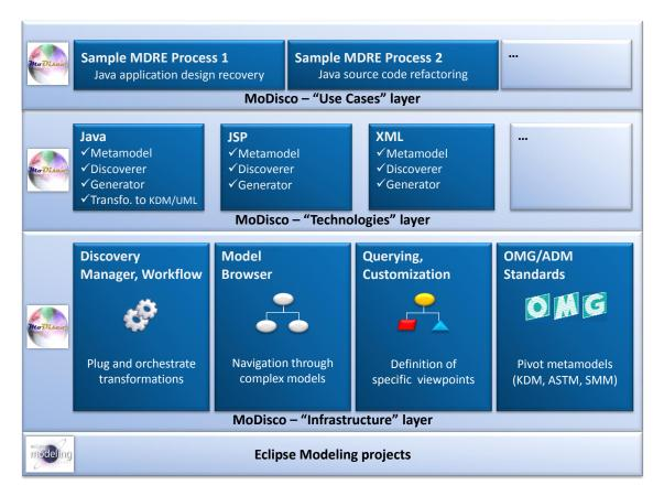
Figure 3.7 – Architecture of the MoDisco framework.
