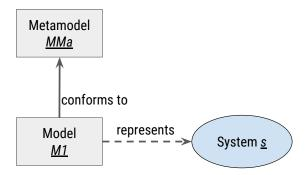
Figure 2.1 – System, model and metamodel.
