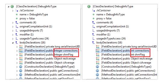
Figure 3.11 – Java model before (left) and after (right) refactoring, using the MoDisco Model Browser to show the effects of the first refactoring.
