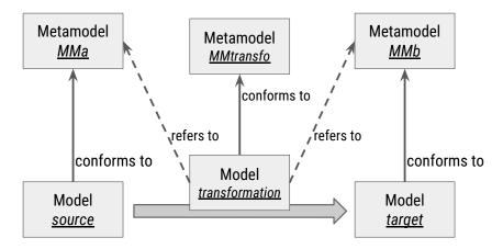
Figure 2.3 – Model-to-model transformation.
