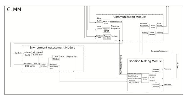
Figure 6.9: CLMM's architecture: information flow between different nodes.
