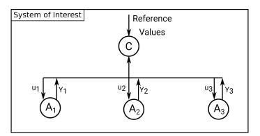
Figure 3.5: Centralized Paradigm: one controller and multiple actuators.
