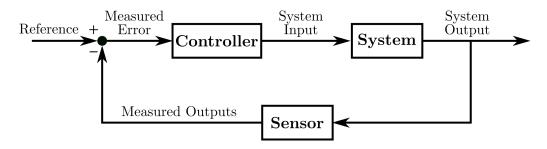
Figure 3.1: Typical system control: a controller computes the system input based on the error between the measured system output and the reference.
