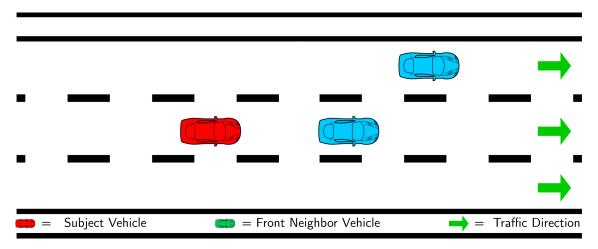
**Figure 6.1:** Overtaking configurations addressed in the CLMM: two or more lanes and same traffic flow direction.
