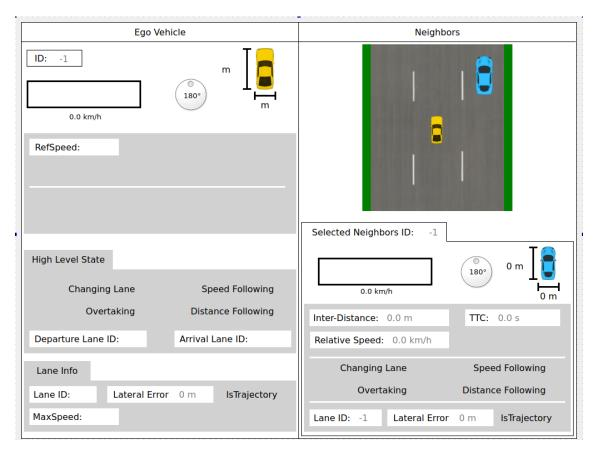
Figure 6.16: Graphical Interface for Monitoring Vehicles' states.
