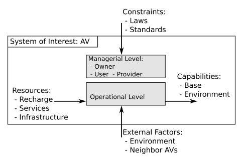
Figure 5.6: Autonomous Vehicle as an independent system: management, functionalities, resources, external factors, and constraints.
