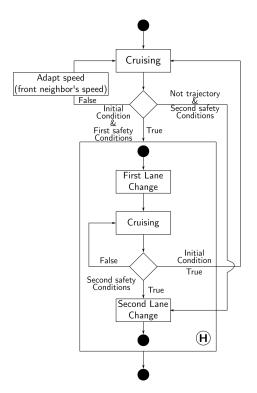
Figure 6.8: Multiple overtaking maneuver flowchart.
