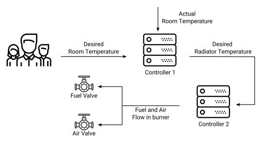
Figure 3.4: Boiler-Room control chain: from high-level to low-level control.
