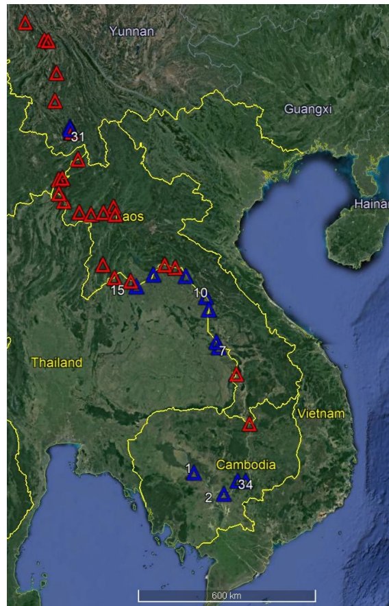
FIGURE 4.9: Locations of 38 virtual stations between ENVISAT/SARAL ground tracks and the Mekong River. Blue presents VSs where altimetry data are good enough to extract surface water height. Figure is created on Google Earth.
