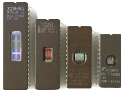
Figure 1.6 – Examples of integrated circuits embedding an electrically erasable ROM that can be erased by shining UV light through the quartz window 16 .
