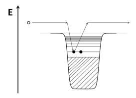
Figure 1.9: Example of a knock-on exchange process that contributes to elastic scattering.
