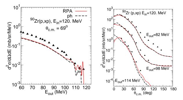
Figure 6.1: Double differential cross sections for (p,xp) off <sup>90</sup>Zr at 120 MeV of incident energy. RPA calculations are displayed as full red curves, uncorrelated particle-hole calculations as black dashed curves. Experimental data from references [2] and [3] are depicted as symbols.
