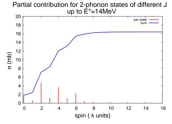
Figure 6.7: Contribution of 2-phonon states (discriminated in terms of their spin) to the total inelastic cross section to 2-phonons up to E\*=14 MeV. The red bars correspond to the total cross section of 2-phonon states with a given spin, and the blue curve is the cumulative sum of their contributions.
