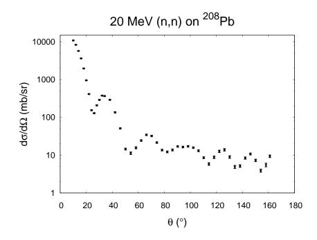
Figure 1.1: Experimental angular distribution [1] for the elastic scattering of neutrons with 20 MeV of kinetic energy off <sup>208</sup>Pb. The cross section for forward angles ( $\theta < 20$ ) is up to 1000 times bigger than for backward angles
