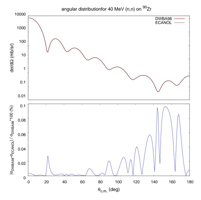
Figure 5.7: Angular distribution and relative difference between the computation done by DWBA98 and our codes for neutron elastic scattering on  $^{90}$ Zr. The maximum radius and the step size used in both codes are rmax=15 fm and h=0.2 fm.
