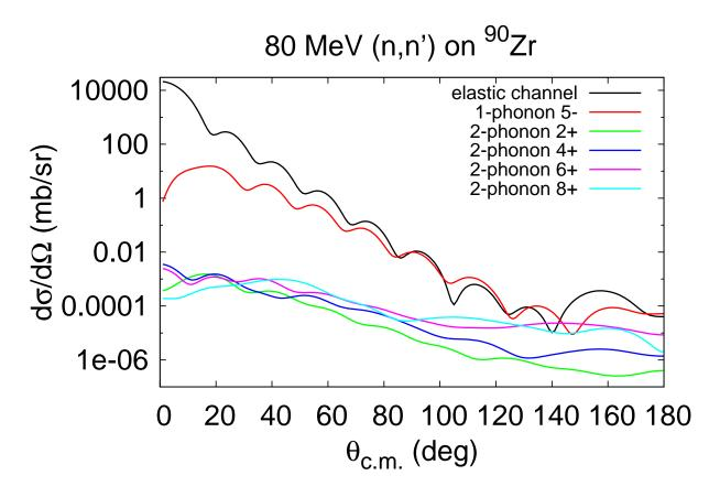
Figure 6.5: Angular distribution to 2-phonon states built by coupling the first, 1-phonon 3<sup>-</sup> state and 5<sup>-</sup> state in <sup>90</sup>Zr for an incident neutron. Here, 2-phonon states are populated exclusively from the 1-phonon 3<sup>-</sup> state.
