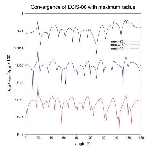
**Figure 5.3:** Relative difference between the angular distribution of a (n,n) reaction on <sup>208</sup>Pb computed by ECIS-06 with a given maximum radius rmax, and the reference with rmax=25 fm. The incident energy is 40 MeV.
