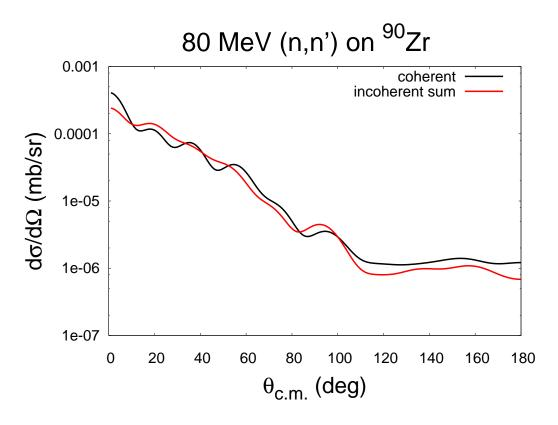
Figure 6.11: Comparison between the angular distribution obtained in a coherent calculation, and the sum of contributions coming from incoherent calculations. The red curve is for the incoherent sum, and the black curve for the coherent calculation.
