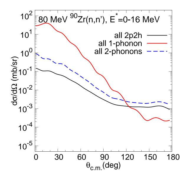
Figure 6.13: Comparison between the angular distribution obtained in a coherent calculation for 1 (red curves) and 2-phonon states (blue curves), and the sum of contributions coming from incoherent calculations of uncorrelated 2p2h (black curves) states. The excitation energies considered in this calculation range from 0 to 16 MeV.
