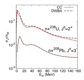
Figure 1.5: Ratios of direct inelastic scattering cross section to direct elastic scattering cross section for incident neutrons on <sup>208</sup>Pb (bottom curve) and <sup>238</sup>U (top curve). Black dashed curves were calculated within the DWBA and red full curves within CC formalism.
