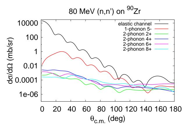
Figure 6.6: Angular distribution to 2-phonon states built by coupling the first, 1-phonon  $3^-$  state and  $5^-$  state in  ${}^{90}$ Zr for an incident neutron. Here, 2-phonon states are populated exclusively from the 1-phonon  $5^-$  state.
