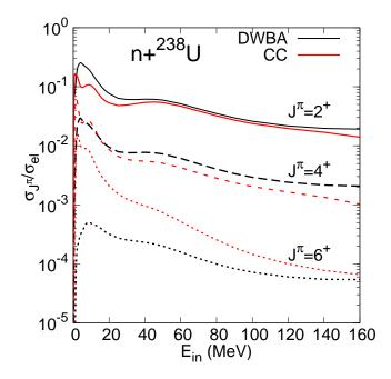
Figure 1.7: Ratios of direct inelastic scattering cross section to direct elastic scattering cross section for incident neutrons on <sup>238</sup>U. Blue curves were calculated within the DWBA and black curves within CC formalism.
