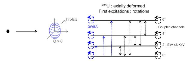
Figure 1.6: Schematic description of the difference between DWBA and CC calculations. Straight arrows depict the existence of a potential connecting one level to another, and circular arrows depict the coupling of partial waves of one level with its other partial waves.
