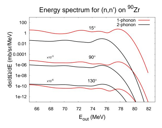
Figure 6.9: Double differential cross section as a function of the emission energy for a (n,n') reaction with an incident energy of 80 MeV on  $^{90}$ Zr. The black curves are the contribution from 2-phonon states up to 20 MeV of excitation energy, the red curves are the contributions from 1-phonon states up to 20 MeV of excitation energy. We display results for emission angles  $\theta = 15$ , 90, 130° in the center of mass frame.
