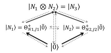
Figure 6.2: Schematic depiction of the couplings leading to an excitation for a 2-step process from excitations of 1-step processes. The full arrows are potentials that are calculated explicitly and included in our calculations, and the dashed arrows represent potentials that are neglected.
