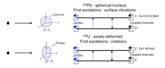
Figure 1.4: Schematic description of the difference between DWBA and CC calculations. Straight arrows depict the existence of a potential connecting one level to another, and circular arrows depict the coupling of partial waves of one level with its other partial waves.
