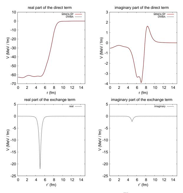
Figure 5.6: Plot of the optical potential for the reaction (n,n) on <sup>208</sup>Pb at an incident energy of 40 MeV in the lab frame, as computed by MINOLOP code. On the upper panels for the direct term, the same calculation done with DWBA code is displayed in red for comparison. The exchange term in the bottom panels is for r = 5 fm and for partial waves  $\{j,l\} = \{\frac{3}{2}, 1\}$
