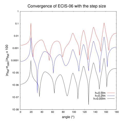
Figure 5.4: Relative difference between the angular distribution of a (n,n) reaction on <sup>208</sup>Pb computed by ECIS-06 with rmax=20 fm, for various values of the step size. The reference calculation is with h=0.01 fm, and the incident energy is 40 MeV.
