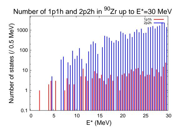
Figure 6.10: Comparison between the number of 1p1h and 2p2h states in <sup>90</sup>Zr for excitation energies below 30 MeV. The red bars correspond to the counting of all 1p1h states and the black bars are for the counting of all 2p2h states, in both cases for an energy bin of 0.5 MeV.
