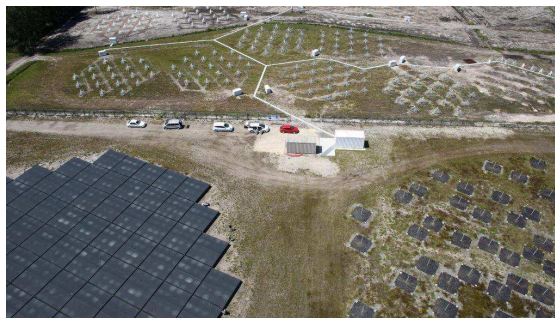
Figure 1.8. Layout of FR606, the French LOFAR station at Nancy. At bottom left are the HBA tiles, bottom right the LBA dipoles, and at the top are some of the NenuFAR tiles.
