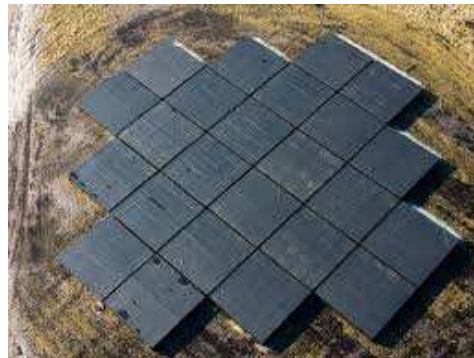
(b) Picture of an HBA tile. Source: Figure 1 of Noorishad et al. (2012)
